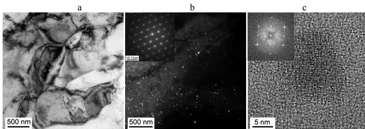
Fig. 4. TEM–structure of alloy 24Zr10Sc alloy after holding at 300 °C during 500 hours: a) polygonized substructure; b),c) nanoparticles of phase  $Al_3(Sc,Zr)$
