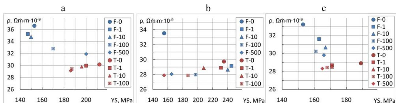
Fig. 5. Relationship between yield strength (YS) and electrical resistance ( $\rho$ ) of cold-rolled aluminium sheets: a) 64Zr; b) 30Sc; c) 24Zr10Sc
