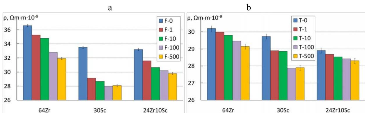
Fig. 3. Electrical resistance ( $\rho$ ) of cold-rolled aluminium sheets (64 Zr, 30Sc and 24Zr10Sc alloys) versus annealing time at 300 °C for 1 up to 500 h: a) scheme F, b) scheme T.
