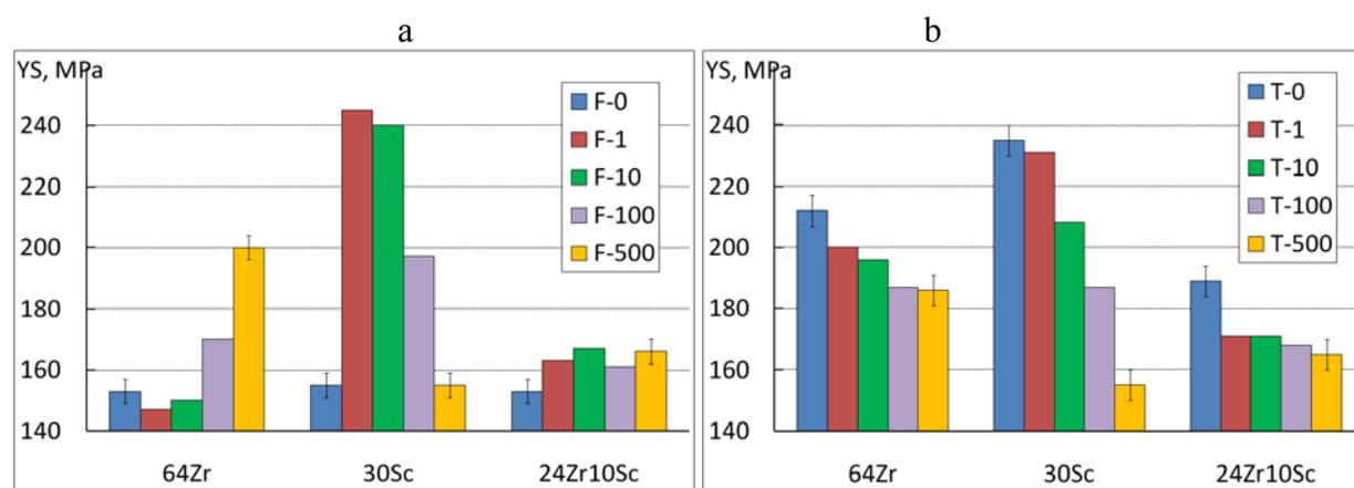
Fig. 2. Yield strength (YS) of cold-rolled aluminium sheets (64 Zr, 30Sc and 24Zr10Sc alloys) versus annealing time at 300 °C for 1 up to 500 h: a) scheme F, b) scheme T.
