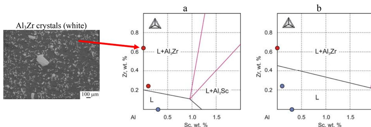
Fig. 1. Isothermal sections of the Al–Sc–Zr phase diagram: a) at 720 °C and b) at 800 °C.
