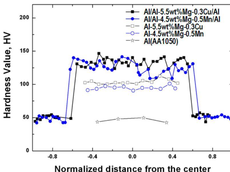
Fig.3 Micro vicker hardness (Hv) of Roll bonded Al/Al-5wt%Mg/Al sheet.
