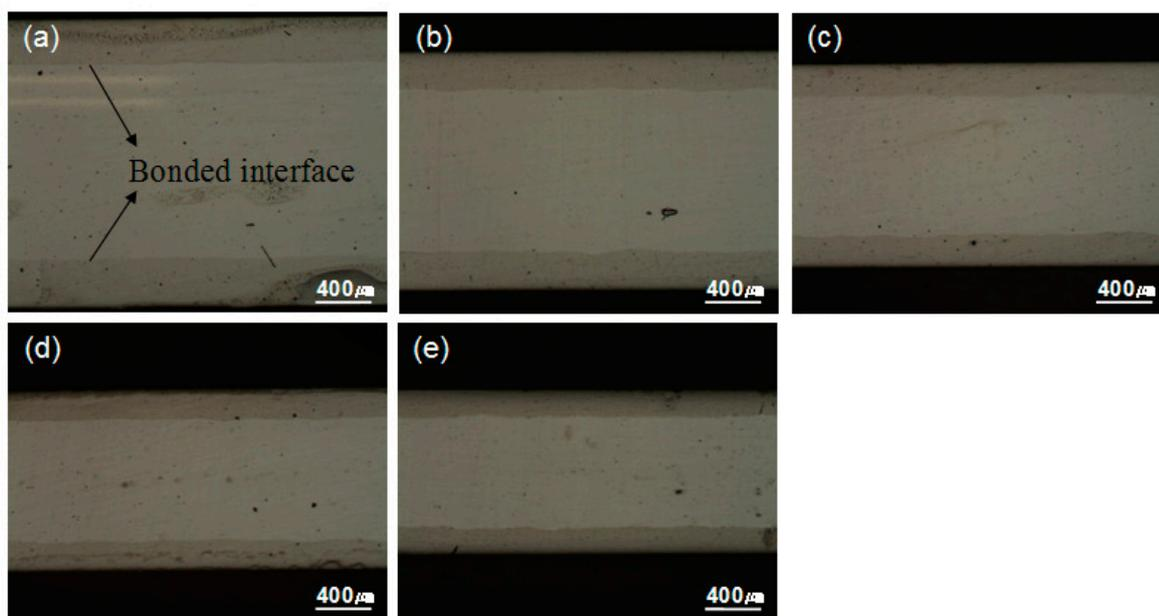
Fig.2 Bonded interface of Al/Al-Mg/Al sheets fabricated by roll bonding under the different rolling reduction; (a) 33%, (b) 43%, (c) 51%, (d) 58 and (e) 63%
