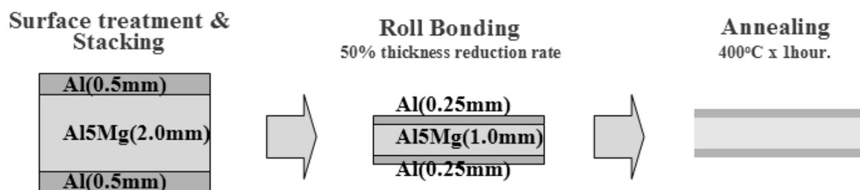
Fig.1 Schematic of roll bonding process for Al/Al-Mg/Al sheets
