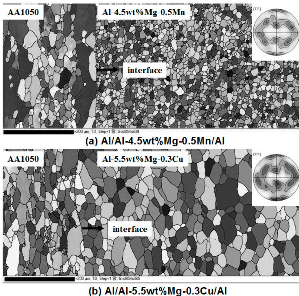
Fig.4 Microstructure of Al/Al-5wt%Mg/Al sheet annealed at 400°C for 1hour; (a) Al/Al-4.5wt%Mg-0.5Mn/Al and (b) Al/Al-5.5wt%Mg-0.3Cu/Al
