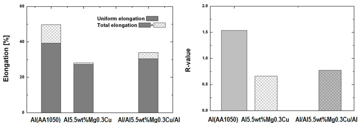
Fig.6 Tensile elongation and plastic strain ratio(R) of Al/Al-5.5wt%Mg-0.3Cu/Al sheet annealed at 400°C for 1hour.
