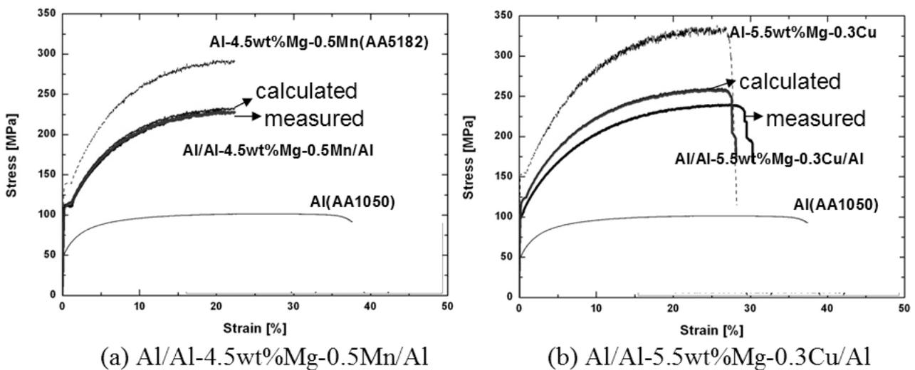
Fig.5 Tensile stress-strain curves of Al/Al-Mg/Al sheet annealed at 400°C for 1hour; (a) Al/Al-4.5wt%Mg-0.5Mn/Al and (b) Al/Al-5.5wt%Mg-0.3Cu/Al
