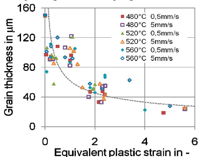
Fig. 8 Coupling of strain with grain thickness for  $\phi=6\text{mm}$  dies.
