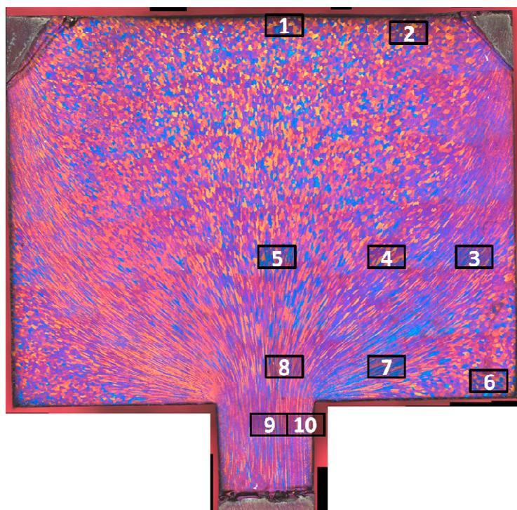
Fig. 6 Overview of the grain structure of a butt, with measured spots.
