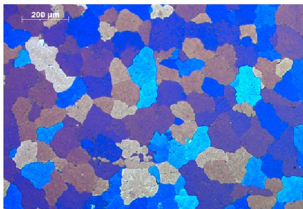
**Fig. 4** Micrograph of etched surface under polarized light.
