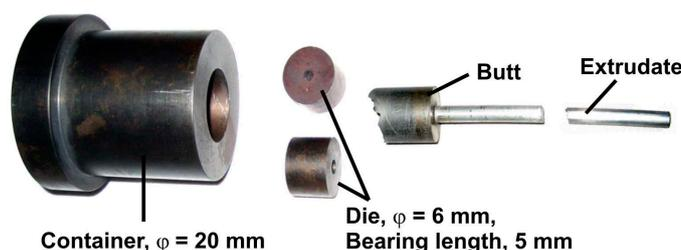
**Fig. 3** Tools: container, butt, die, strand.
