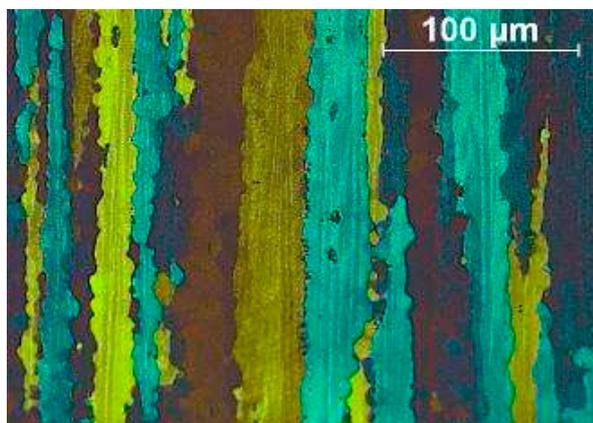
**Fig. 1** Micrograph of En AW-6082, in the middle of an extruded strand.
