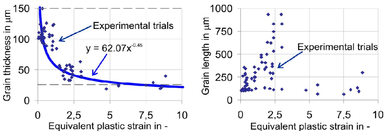
Fig. 9 a) Coupling of strain with grain thickness; b) Coupling of strain with grain length.
