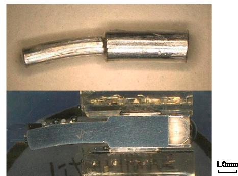
Fig. 4 Samples of micro-pins obtained during forward-backward micro-extrusion
