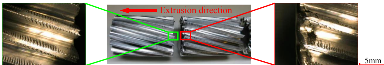
Fig.8 The photograph of the shape after extrusion (30mm-division billet)
