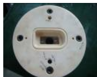
Fig. 5. Machined resin tooling.
