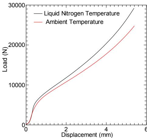
Fig. 2 Load–displacement curves during compression at ambient and liquid nitrogen temperatures.
