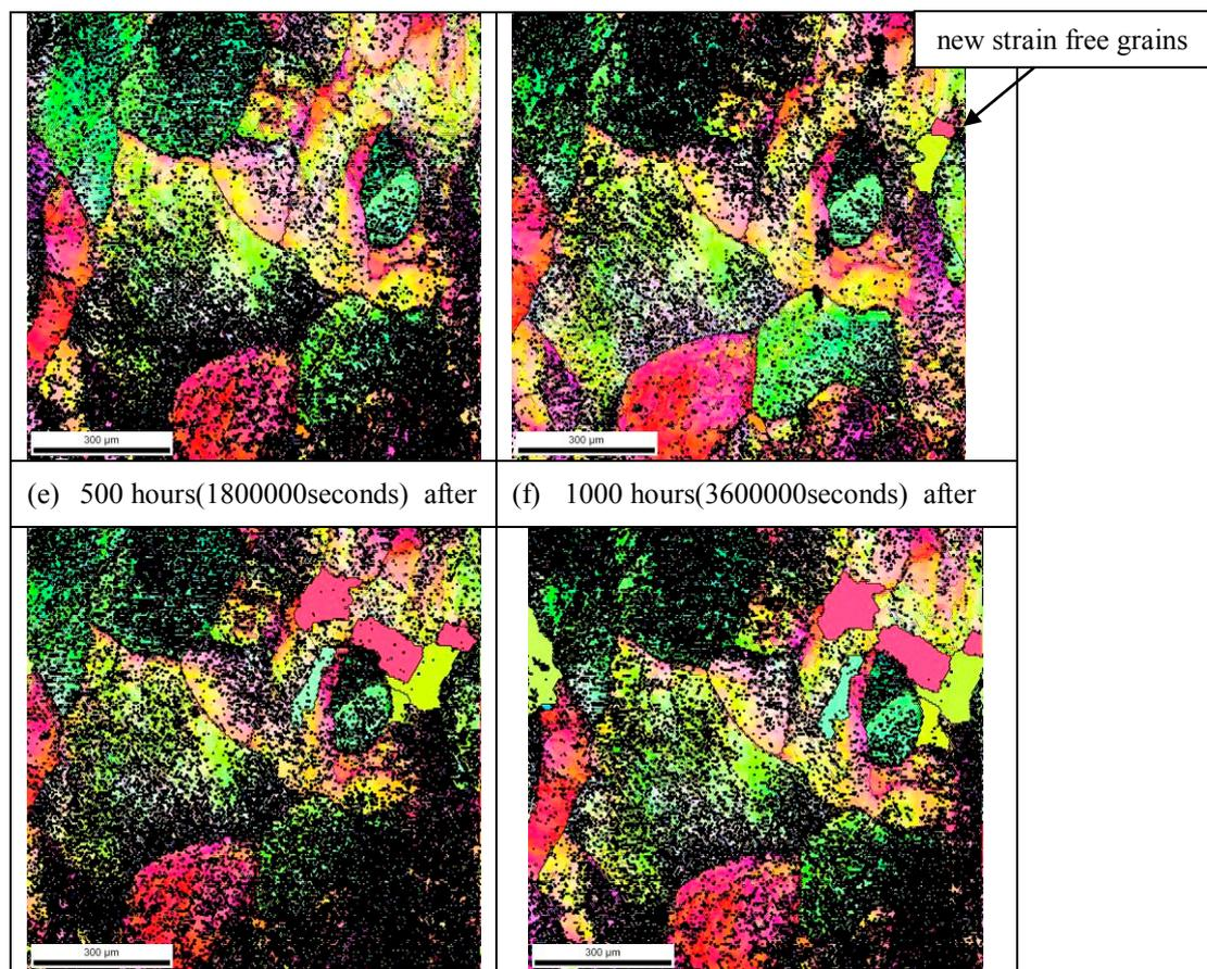
Fig. 3 Microstructure change at AT after AT compression.
