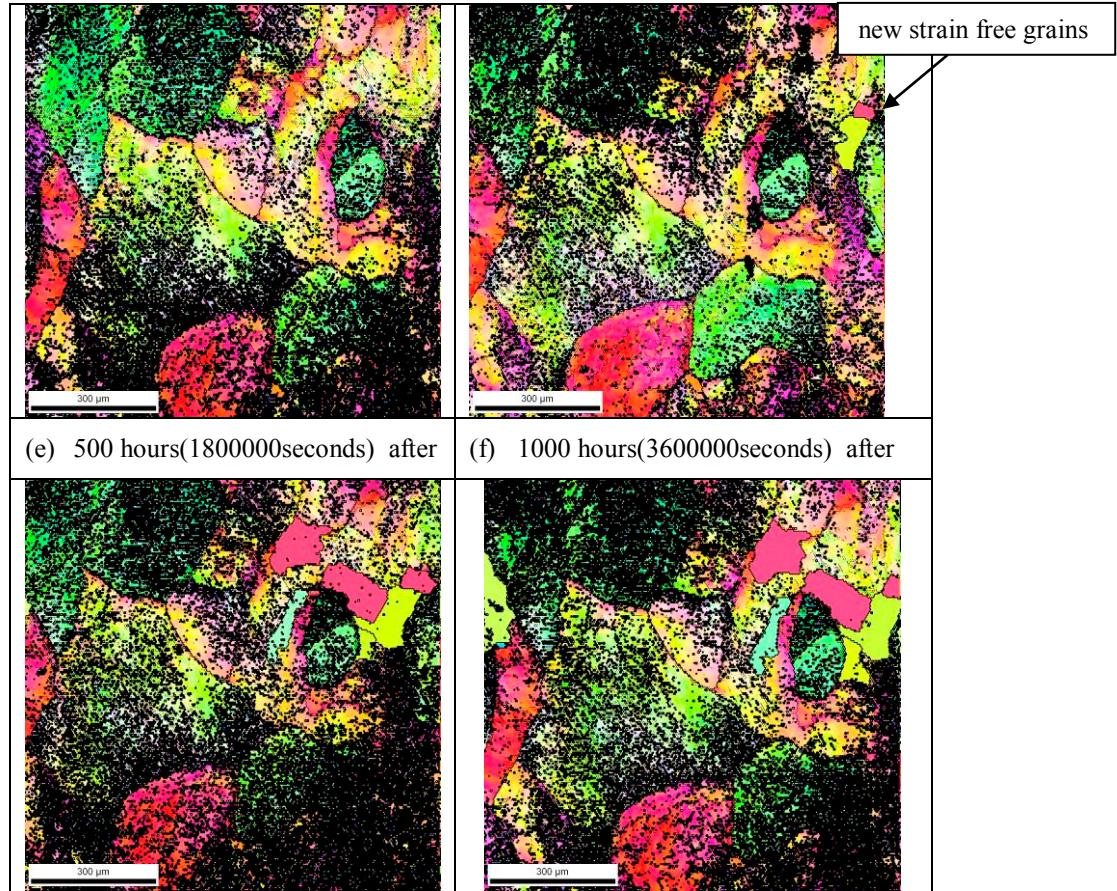
Fig. 3 Microstructure change at AT after AT compression.
