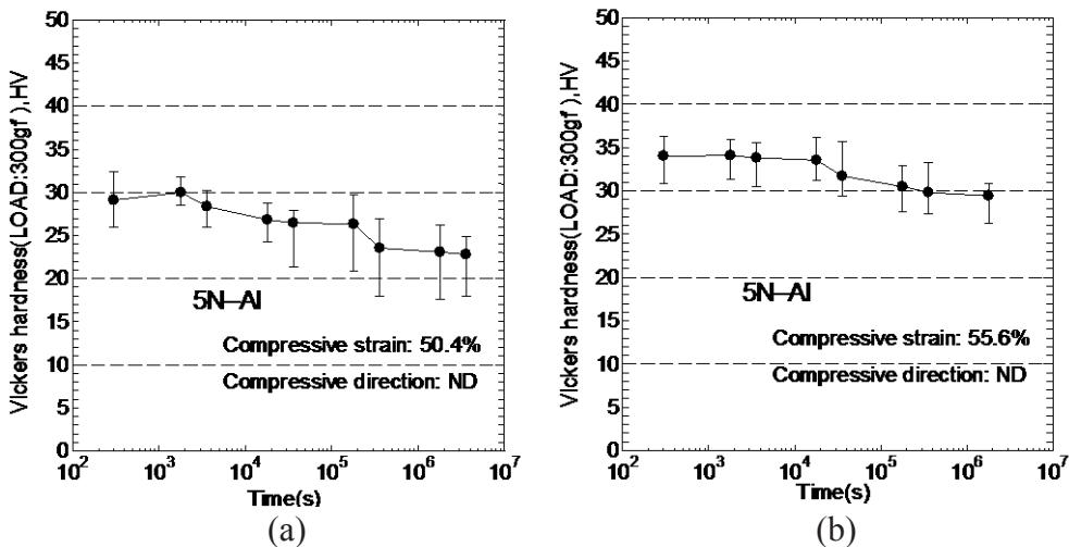
Fig. 1 Change in Vickers hardness at ambient temperature after compression at (a) ambient and (b) liquid nitrogen temperatures.
