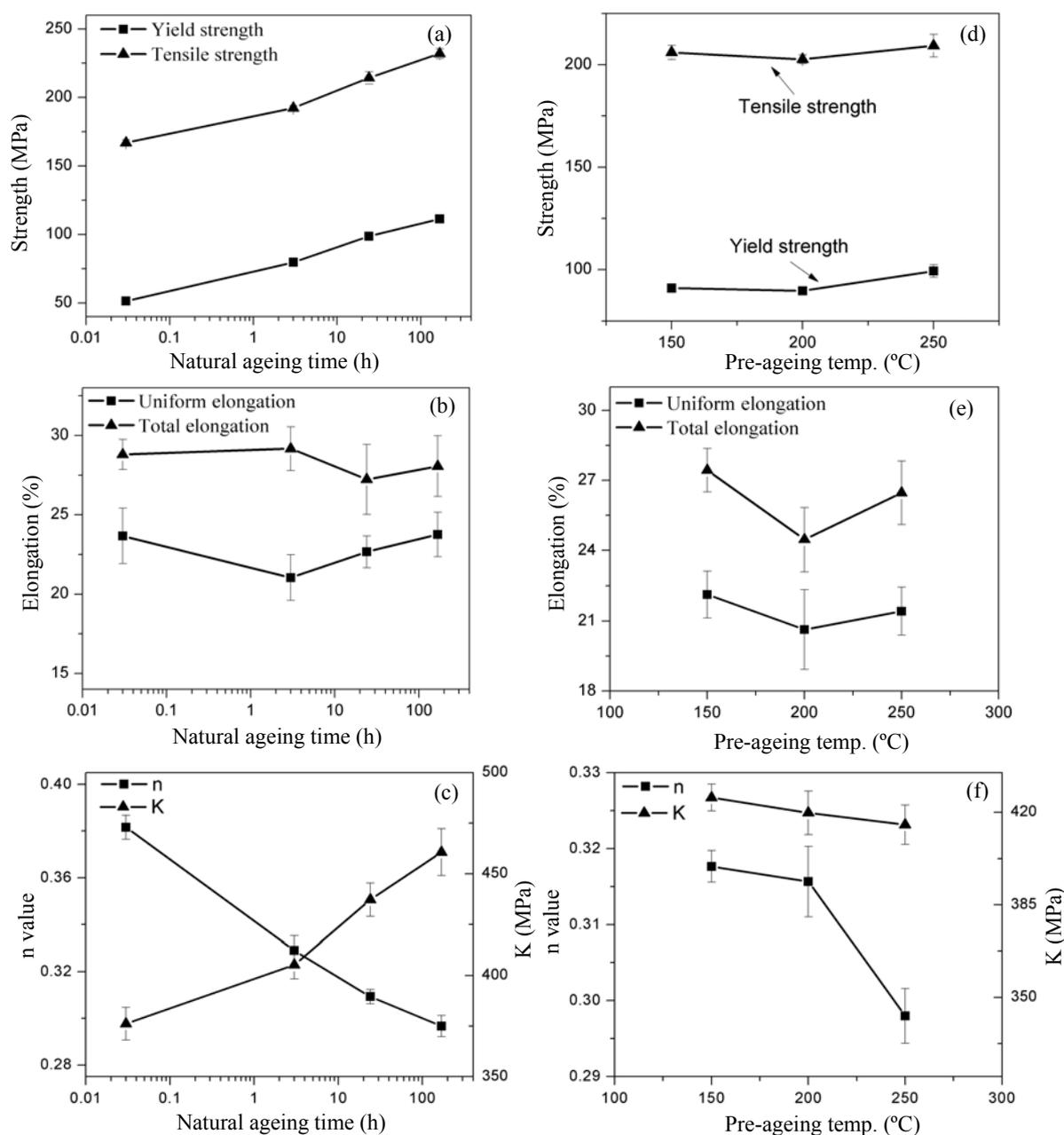
Fig. 1: Effect of natural ageing on (a) strength, (b) elongation and (c) values of  $n$  and  $K$ , and pre-ageing temp. on (d) strength, (e) elongation and (f) values of  $n$  and  $K$
