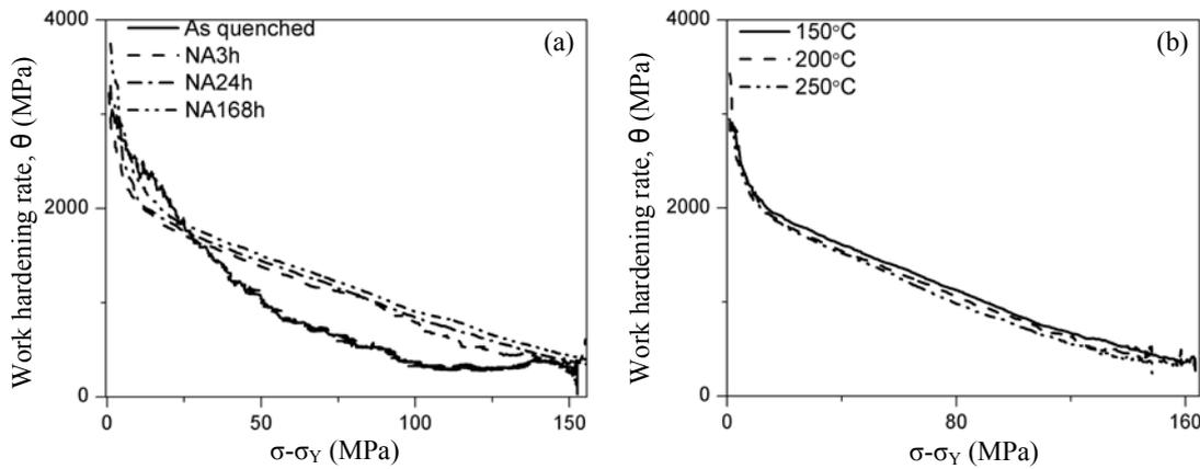
Fig. 3: The instantaneous work-hardening rate vs plastic flow stress for (a) as-quenched and naturally aged and (b) pre-aged 6016 samples
