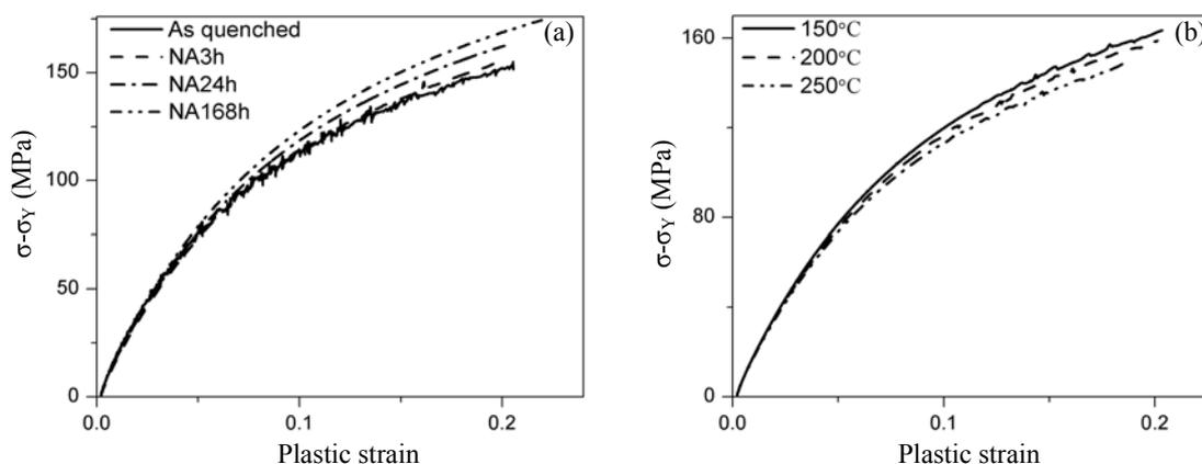
Fig. 2: Plastic stress-strain curves for (a) as-quenched and naturally aged and (b) pre-aged samples
