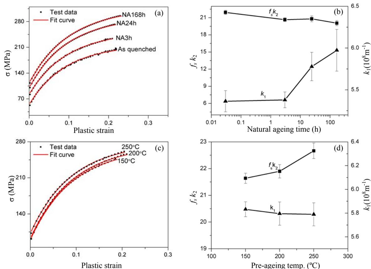
Fig. 4: Stress-strain curves and model parameters for (a, b) naturally aged and (c, d) pre-aged conditions
