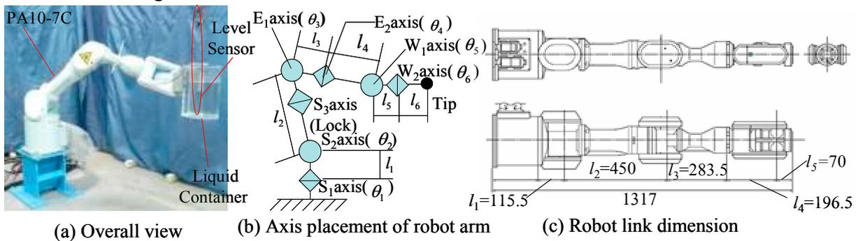
Fig.1 Complete setup of the liquid transfer system
