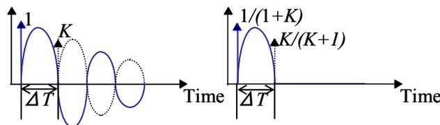
Fig.3 .Principle of input shaping
