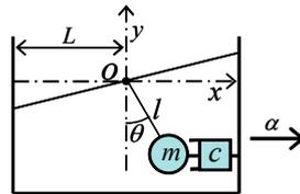
Fig.2 Pendulum model of one-mode sloshing
