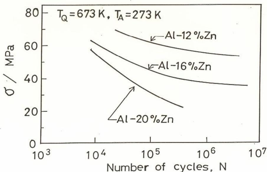
Fig.3 Plot of stress amplitude against number of stress cycles for alloys aged at 273K after quenching from 673K.
