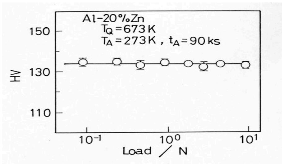
Fig. 2 Dependence of hardness number on the load for the Al-20%Zn alloy aged at 273K for 90ks after quenching from 673K.
