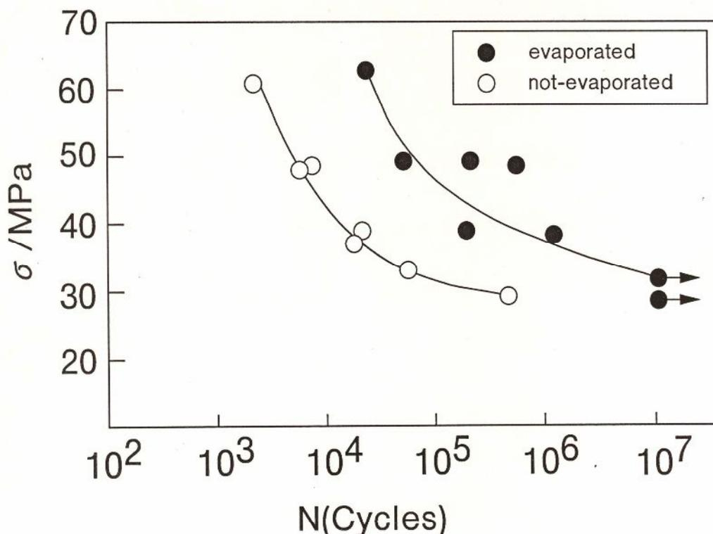
Fig.4 Effect of evaporated Al layer on  $\sigma$  - N curve of Al-20%Zn alloy aged at 273K for 90ks after quenching from 673K.
