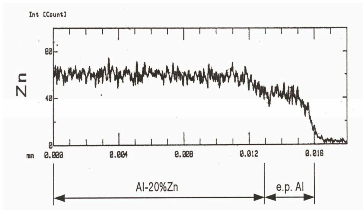
Fig. 5 Variation of Zn concentration with the distance from surface of Al evaporated and heat treated Al-20%Zn alloy specimen.
