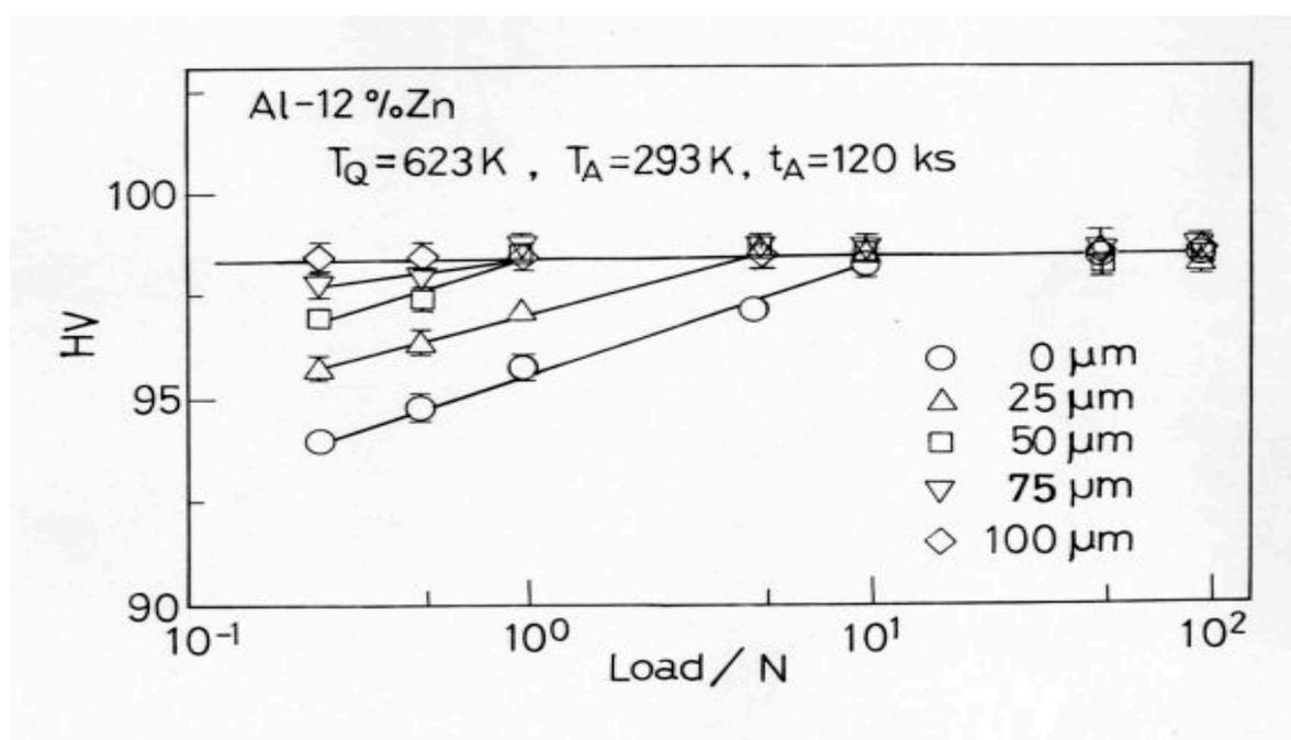
Fig.1 Variation with indentation load of hardness of the Al-12%Zn specimen aged at 293K for 120ks after quenching from 623K. Surface layer was successively removed layer by layer, each 25  $\mu\text{m}$  in thickness, and the load dependence was measured after each removal.
