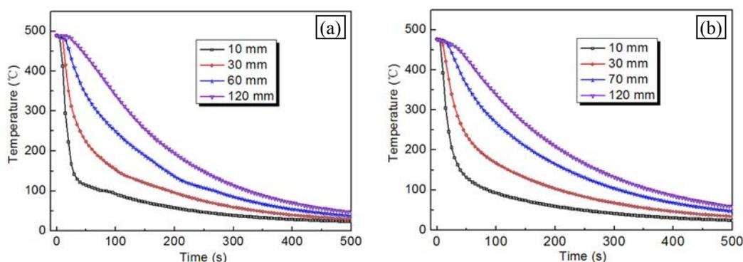
Fig.2 Cooling curves at different locations along the Jominy end quench specimen. (a) AA2124; (b) AA7050
