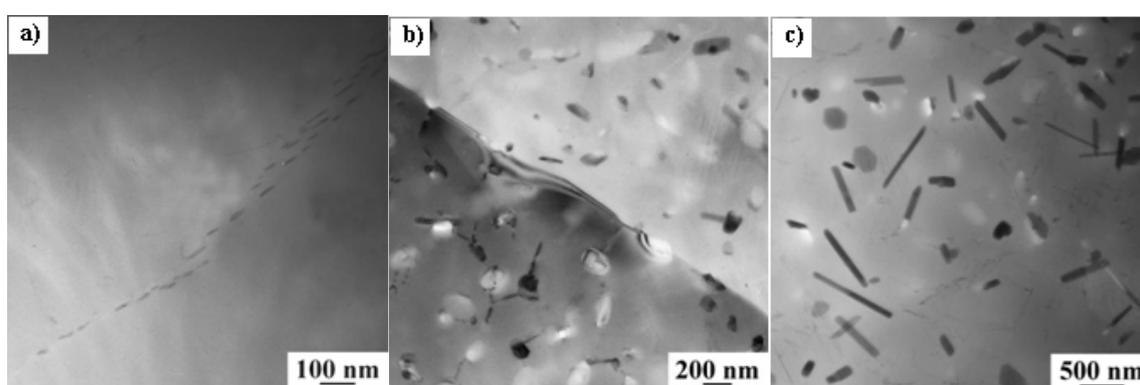
Fig.5 TEM images of precipitates of the as-quenched AA 7B04 at different locations from quenched end. (a) 5mm; (b) 40mm; (c) 100mm
