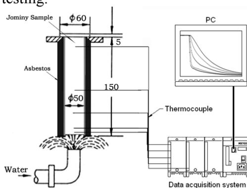
Fig.1 Schematic of the Jominy end quench test kit
