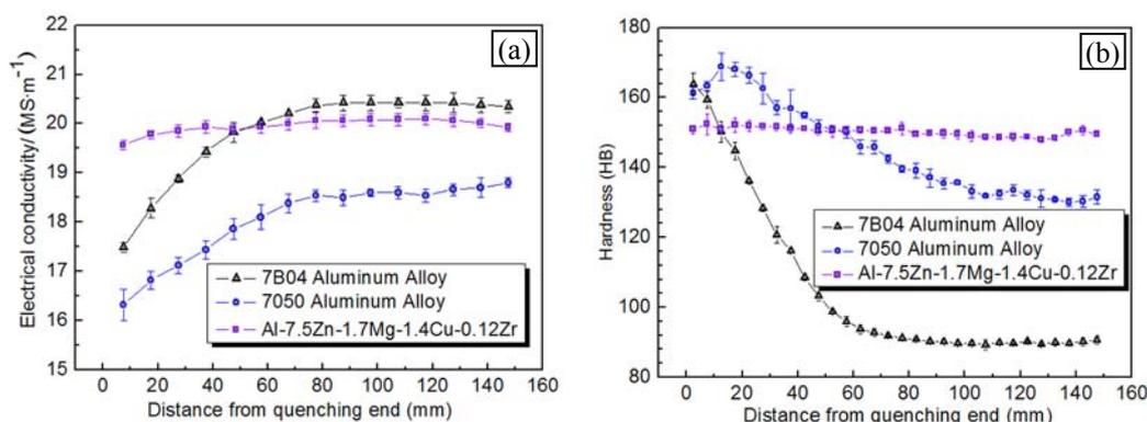
Fig.4 (a) Electrical conductivity in as-quenched and (b) hardness in as-aged as function of Jominy distance for selected 7000 series Al alloys
