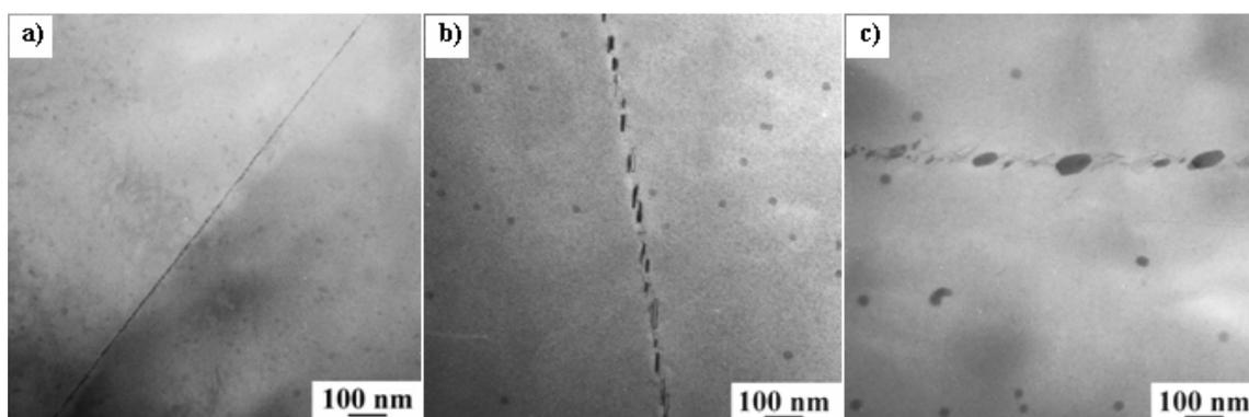
Fig.6 TEM images of precipitates of the as-quenched Al-7.5Zn-1.7Mg-1.4Cu-0.12Zr alloy at different locations from quenched end. (a) 5mm; (b) 40mm; (c) 100mm
