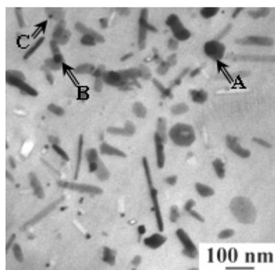
Fig.7 TEM image of quench-induced precipitates inside partial grain of Al-7.5Zn-1.7Mg-1.4Cu-0.12Zr alloy at 100 mm distance from quenched end
