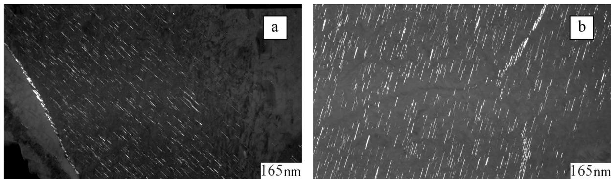
Fig. 3 – Dark-field image of  $\Omega'$ -phase plates with habitus  $(111)_\alpha$ :
