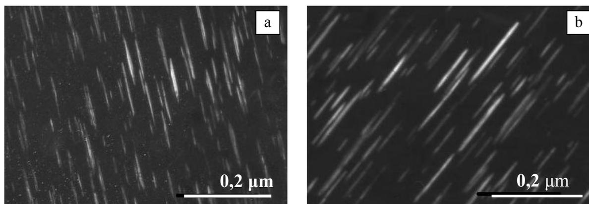
Fig. 4 - Dark-field image of  $\Omega'$ - phase plates: a) T1; b) T1+ 150°C, 1000 h
