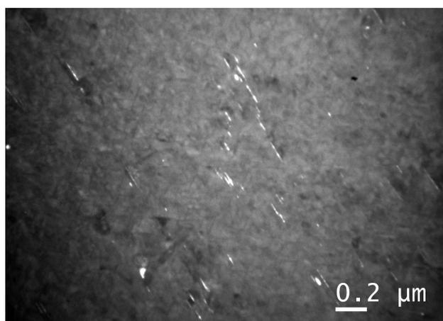
Fig. 6 - Dark-field image of  $\theta'$ -phase (T1 +150°C, 1000 h)
