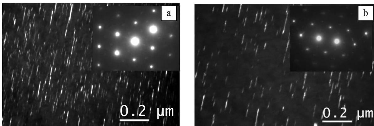
Fig. 5 - Dark-field image of  $\Omega'$ - phase in forgings:
