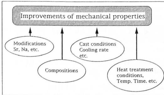
**Fig.1 Schematic illustration showing the improvement of the mechanical properties of the A356 casting alloy.**
