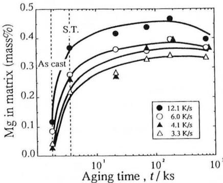
**Fig.6** Change of Mg concentrations in the matrix by various cooling rates.
