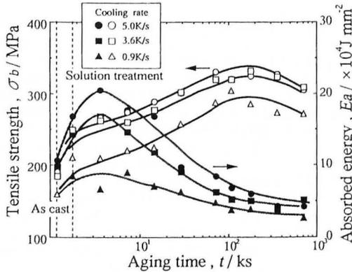
**Fig.5** Aging response of the tensile strength and Charpy impact properties of the A356 alloy specimens cast under various cooling rates.
