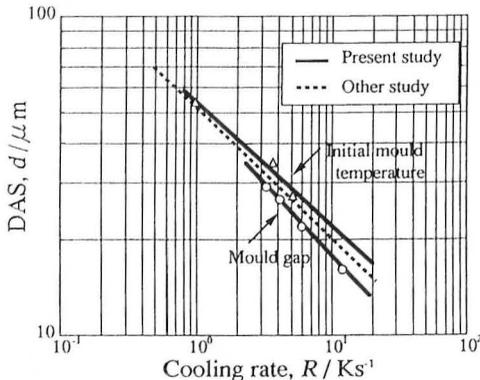
**Fig.2 Effect of cooling rate on dendrite arm spacings.**
