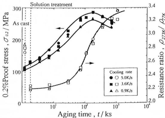
**Fig.4** Aging response of the resistance ratio and the proof stress for the specimens cast under various cooling rates.
