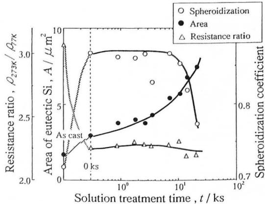
**Fig.3 Effect of solutioning temperature and time on the redissolution of the solutes, and shape or size of eutectic.**
