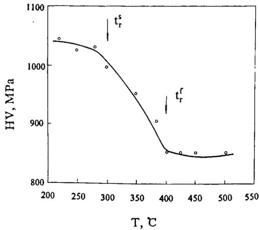
Fig.1 Hardness vs annealing temperature curve holding time 60 min
