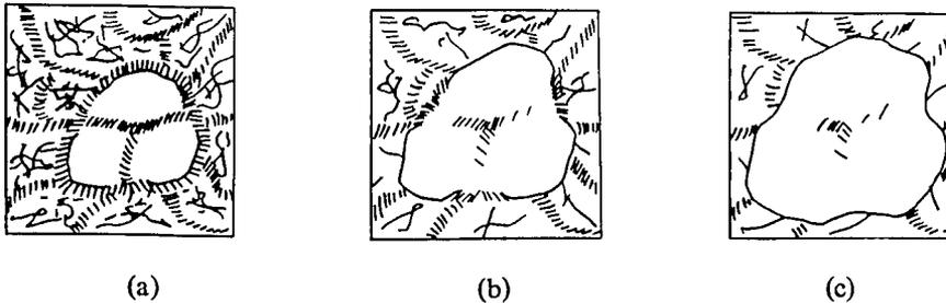
Fig.3 Subgrain coalescence accompanied by subgrain growth
