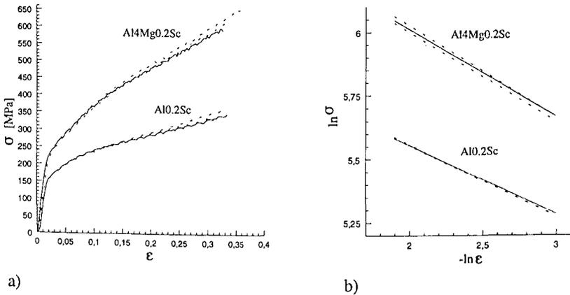
Figure 4. Stress/strain and mean  $\ln \sigma / \ln \epsilon$  -curves for the compression test specimens.
