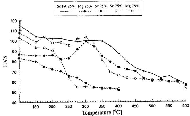
Figure 5 Hardness measurements from isochronal annealed specimens.
