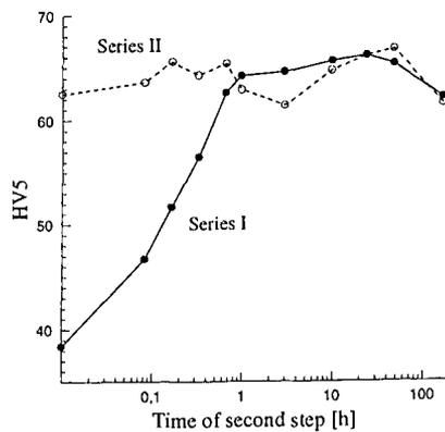
Figure 3. Hardness measurements from second step of two-step ageing.
