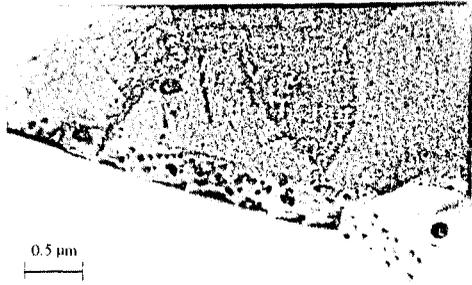
Figure 8. Particles of  $\text{Al}_3\text{Sc}$  on the recrystallization front.
