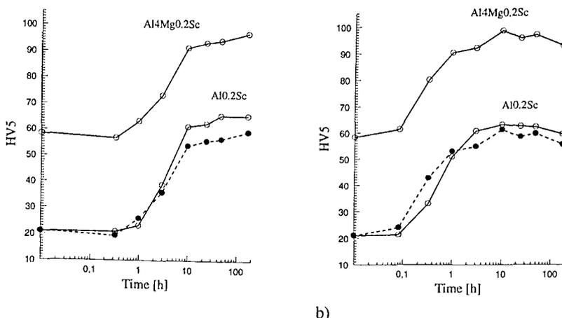
Figure 1 Hardness measurements from age hardening at a) 250 and b) 300°C.
