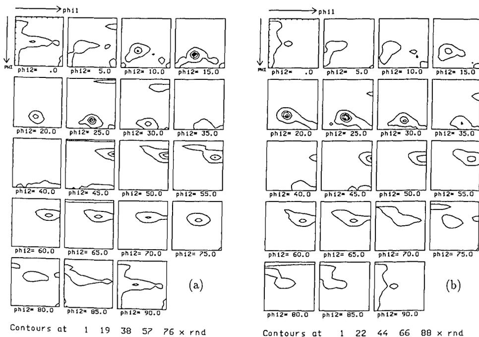
Figure 5: ODFs simulated for a strain  $\varepsilon_{vM} = 2.0$  starting from the experimental texture (a) Full Constraints model. (b) Relaxed Constraints model.
