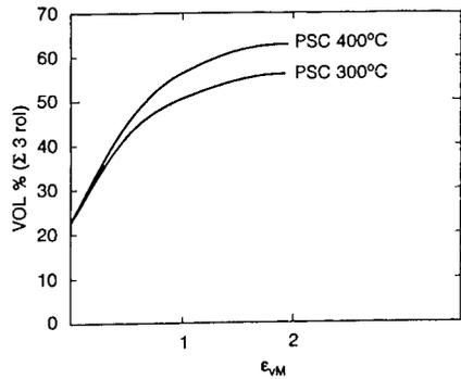
Figure 2: Development of the total volume fraction of the three rolling texture components (copper, S, brass) during PSC
