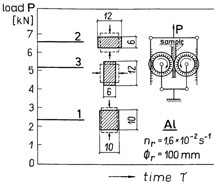
Figure 1. Mechanical characteristics of aluminum during monotonic and cross-rolling. Dimensions of the roll pass designs, scheme of the testing and measuring device are also shown.
