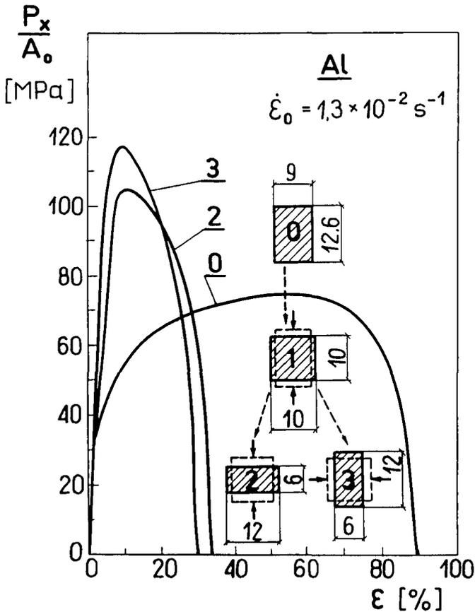
Figure 4. Tensile curves of monotonically (line 2), cross-rolled (line 3) and virgin aluminum.
