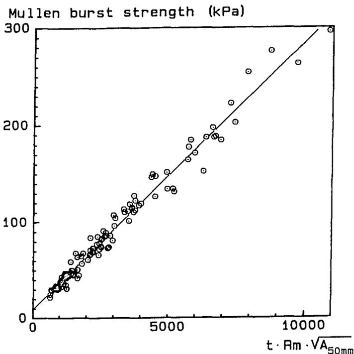
Figure 3. The relation between the Mullen burst strength,  $p$ , and the foil gauge,  $t$ , tensile strength,  $R_m$ , and elongation at fracture,  $A_{50mm}$ . The straight line is a representation of  $p = 8.8 + 0.0277 \cdot t \cdot R_m \cdot A^{1/2}$ , with  $t$  in  $\mu\text{m}$ ,  $R_m$  in MPa and  $A_{50mm}$  in %.
