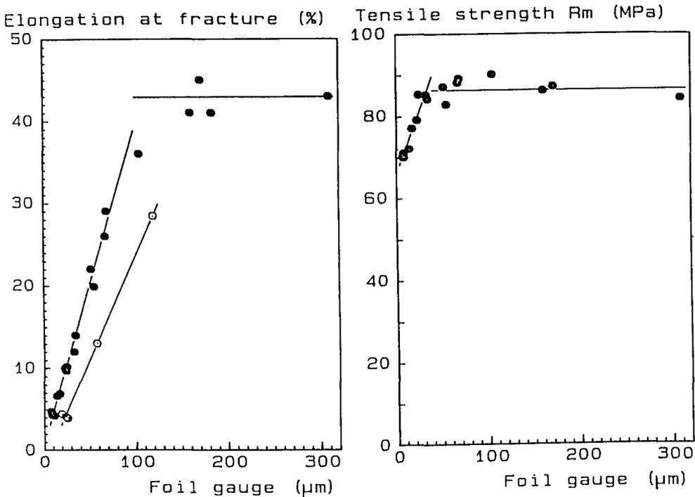
Figure 4. The influence of foil gauge on the tensile properties of strip cast, soft annealed AA8111 foil. Filled circles: grain size 15  $\mu\text{m}$ . Open circles: grain size 40 - 60  $\mu\text{m}$ .
