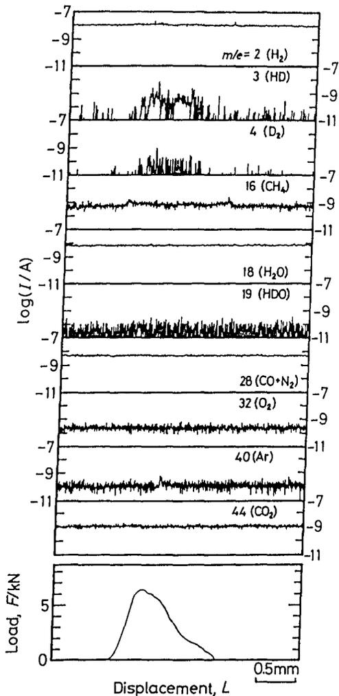
Figure 5. Correlation between a load-displacement curve and gas evolution behavior of an Al-Mg specimen strained in a vacuum of  $2.3 \times 10^{-7}$  Pa at ambient temperature.
