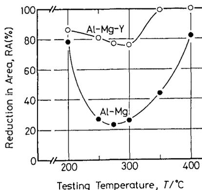
Figure 3. Reduction in area vs. testing temperature curves of Al-5.1%Mg and Al-5.1%Mg-0.04%Y alloys.
