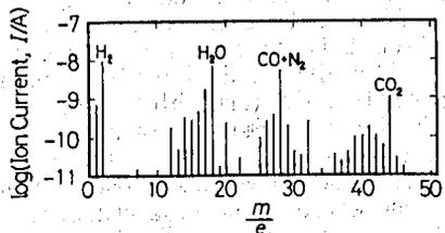
Figure 2. Result of residual gas analysis in the ultra high vacuum chamber of the equipment shown in Fig. 1. Pressure is 2.3x10<sup>-7</sup>Pa.
