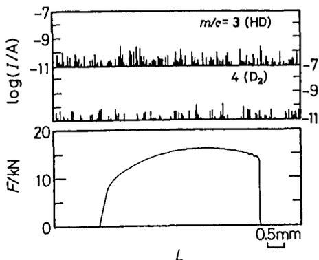
Figure 7. Correlation between a load-displacement curve and gas evolution behavior of an Al-Mg-Y specimen strained in a vacuum of  $2.3 \times 10^{-7}$  Pa at ambient temperature.
