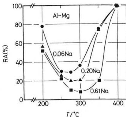
Figure 7. Effect of sodium on reduction in area of an Al-Mg alloy.
