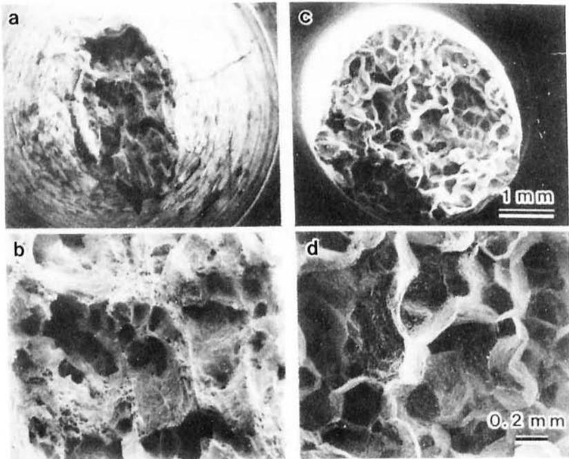
Figure 1. SEM fractographs of the Al-4.7Mg-0.03Y specimens tested at 300°C and at a strain rate of  $8.3 \times 10^{-4} \text{s}^{-1}$ . Gage length and diameter are 10 and 4mm, respectively. Grain size is 0.3mm. Reduction in area: 67%(a) and 33%(c). Sodium content: 0.14massppm(a) and 0.35massppm(c). (b,d): magnified images of (a,c), respectively.
