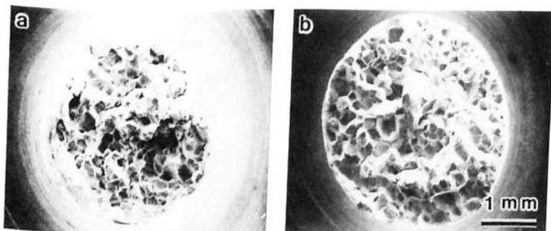
Figure 5. SEM fractographs of Al-Mg-Y specimens containing sodium of 0.50 (a) and 0.60ppm (b) tested at 275°C.
