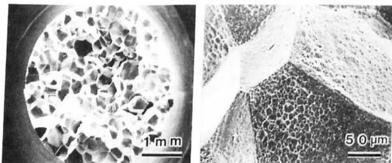
Figure 8. SEM fractographs of an Al-Mg specimen containing 0.61ppm sodium.
