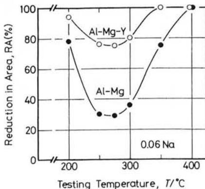
Figure 2. Reduction in area vs. testing temperature curves of Al-5%Mg and Al-5%Mg-0.04%Y alloys containing 0.06ppm sodium.
