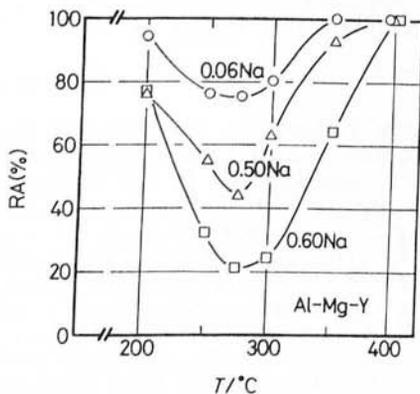
Figure 4. Effect of sodium on reduction in area of an Al-Mg-Y alloy.
