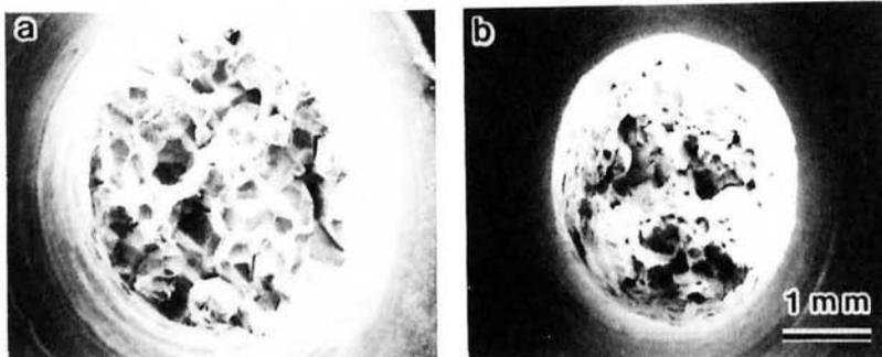
Figure 3. SEM fractographs of Al-Mg (a) and Al-Mg-Y (b) specimens tested at 275°C. Sodium content is 0.06ppm.
