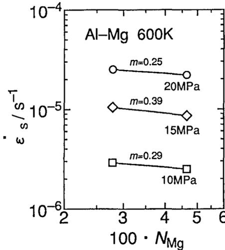
Figure 5. The steady-state creep rate of Al-Mg solid solutions in a high concentration range (near the solubility limit) as a function of concentration. The concentration exponent is obviously smaller than that in low concentration alloys. All samples have similar grain size,  $\sim 0.3\mu\text{m}$ .
