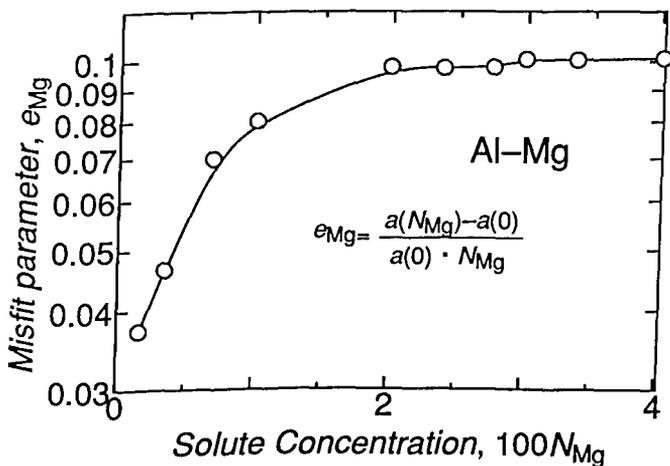
Figure 4. The size misfit parameter estimated from the concentration dependence of the lattice parameter which are quoted from reference[9]. Lattice parameters used for calculations are those reported by Poole and Axion(1952).
