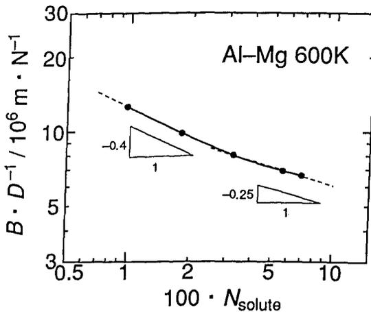
Figure 6. The mobility of dislocations  $B$  compensated by diffusion coefficient  $D$  as a function of solute concentration. The concentration effect on the mobility decreases as increasing solute concentration.
