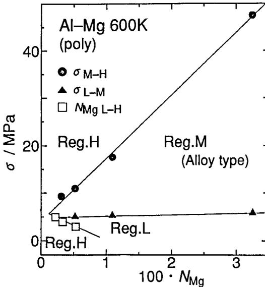
Figure 3. Regions classified and the transition conditions between regions. Type-A behavior is observed in bounded conditions and are not observed in Al-0.1mol%Mg.
