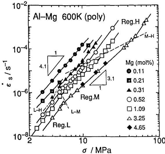
Figure 1. The steady-state creep rate of Al-Mg solid solution alloys at 600K as a function of applied stress.
