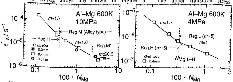
Figure 2. The concentration dependence of the steady-state creep rate of Al-Mg alloys at 10MPa(a) and 4MPa(b). The slope indicates the concentration exponent  $m$ , and decreases with increasing concentration.
