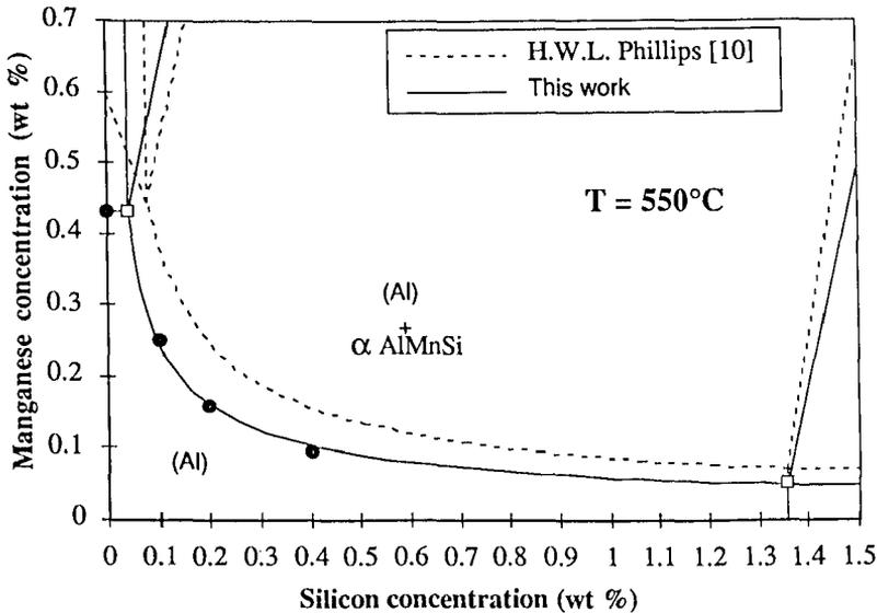
Figure 2: Comparison between the solvus from Phillips[10] and the present work.
