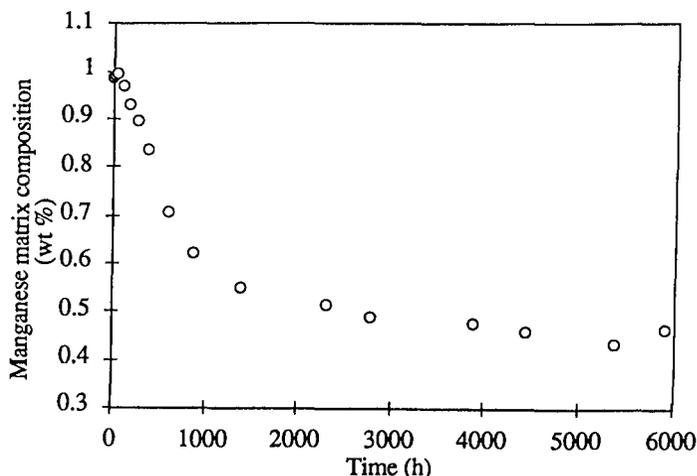
Figure 1: Evolution of the manganese matrix composition of Al-1wt% Mn at 550°C (accuracy of the measurements  $\pm 0.02$  wt %).
