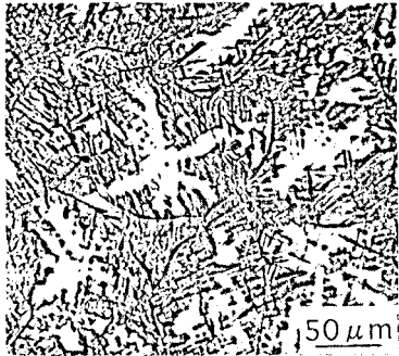
Fig.7 Nonuniform precipitation structure in Al-9.45%Mg-0.13%Ti alloy aged at 453K for 25h.
