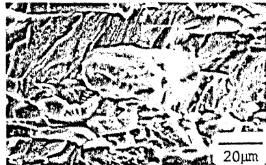
a) PCS, \Delta K = 8 \text{ MPa} \cdot \text{m}^{1/2} b) TMT, \Delta K = 4.9 \text{ m/cycle} Fig. 12: 7475, UA, Fracture surfaces (SEM), NaCl Sol., da/dN = 10^{-8} \text{ m/cycle} , R = 0.1
