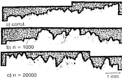
Fig. 3: X-7075, CG, Profiles, R = 0.1,  $da/dN \approx 10^{-9}$  m/cycle (3)
