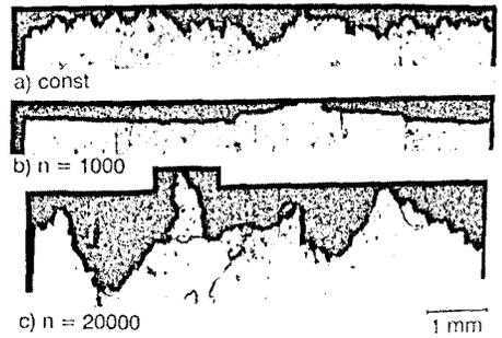
Fig. 4: X-7075, CG, Profiles, R = 0.5,  $da/dN \approx 10^{-9}$  m/cycle (3)
