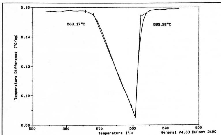
Figure 3. DTA-measurement of the sprayformed Al/36Si alloy.
