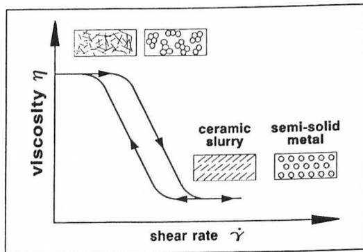
Figure 1. Viscosity as a function of shear rate of thixotropic materials /1/.
