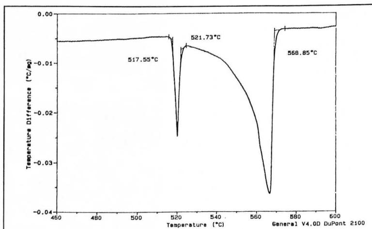
Figure 4. DTA-measurement of the sprayformed Al/36Si/5Cu alloy.
