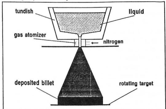
Figure 2. Schematic arrangement of Osprey compaction process /6/.
