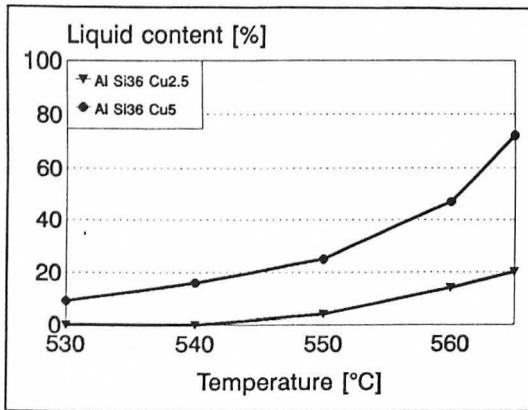
Figure 8. Amount of liquid as a function of the temperature of heat treatment.
