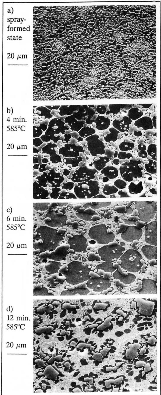
Figure 5 a-d. Microstructures of the spray-formed Al/20Si after heat treatment in the semi-solid state.
