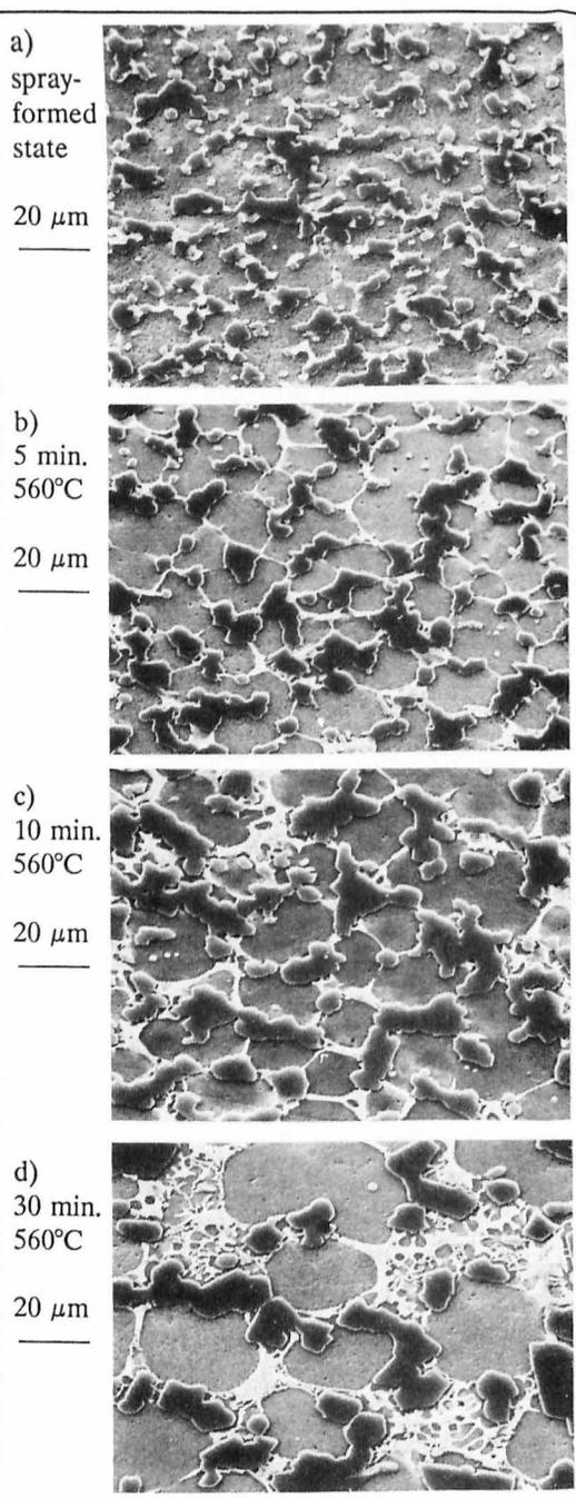
Figure 7 a-d. Microstructures of the spray-formed Al/25Si/5Cu alloy after heat treatment in the semi-solid state.
