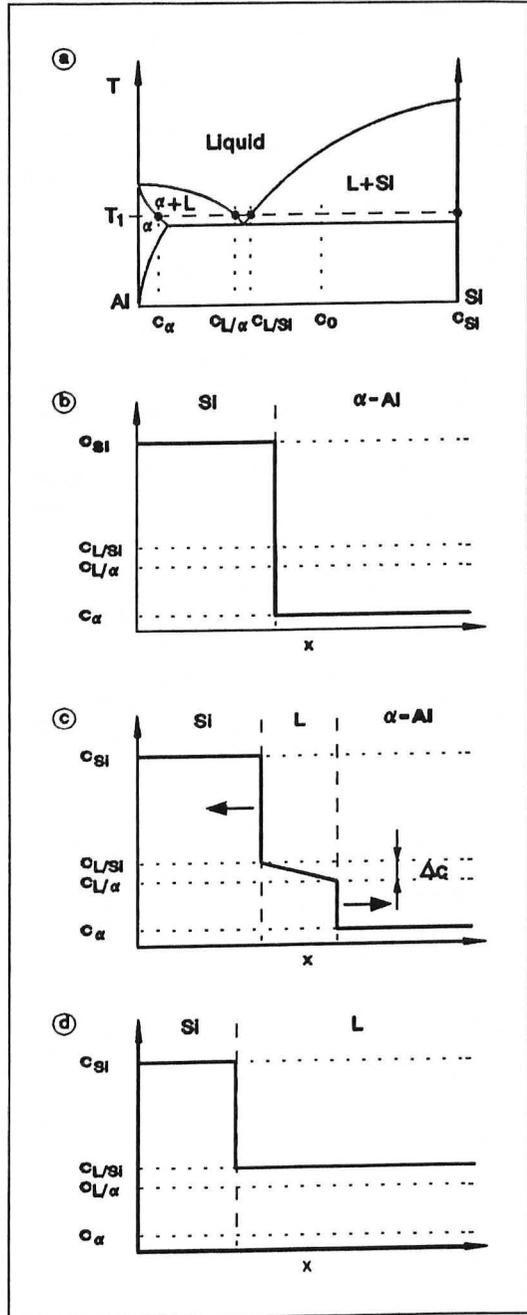
Figure 6 a-d. Schematic model of the remelting process.
