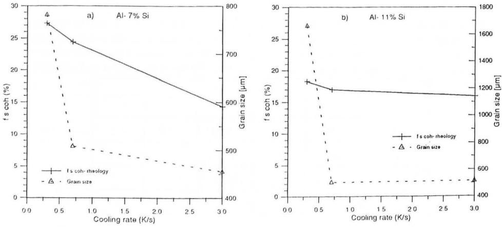
Figure 4. Effect of cooling rate on dendrite coherency, determined rheologically, and grain size in a) Commercial Al-7%Si-0.05%Ti and b) Commercial Al-11%Si-0.05%Ti.
