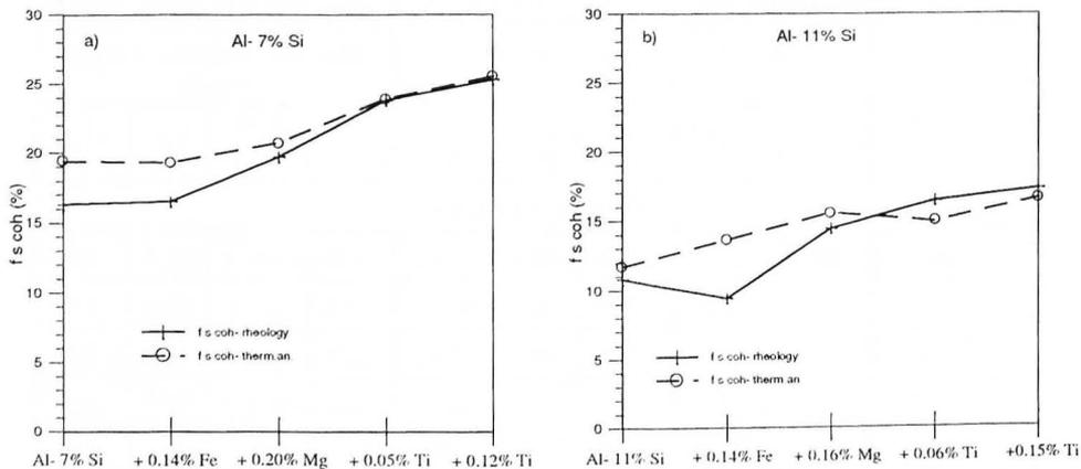
Figure 6. Effect of successive additions of iron, magnesium,  $\sim 0.05\%$  Ti as Al-5Ti-1B and  $\sim 0.15\%$  Ti in a) pure Al- 7% Si and b) pure Al- 11% Si. The level of additions is chosen to reproduce the composition of the commercial alloys.[0.7 K/s].
