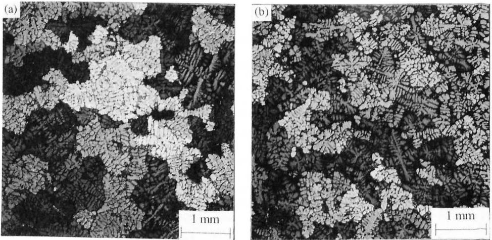
Figure 3. Micrographs showing the effect of grain refinement in commercial Al-7% Si. a) not grain refined and b) grain refined with 0.20% Ti.
