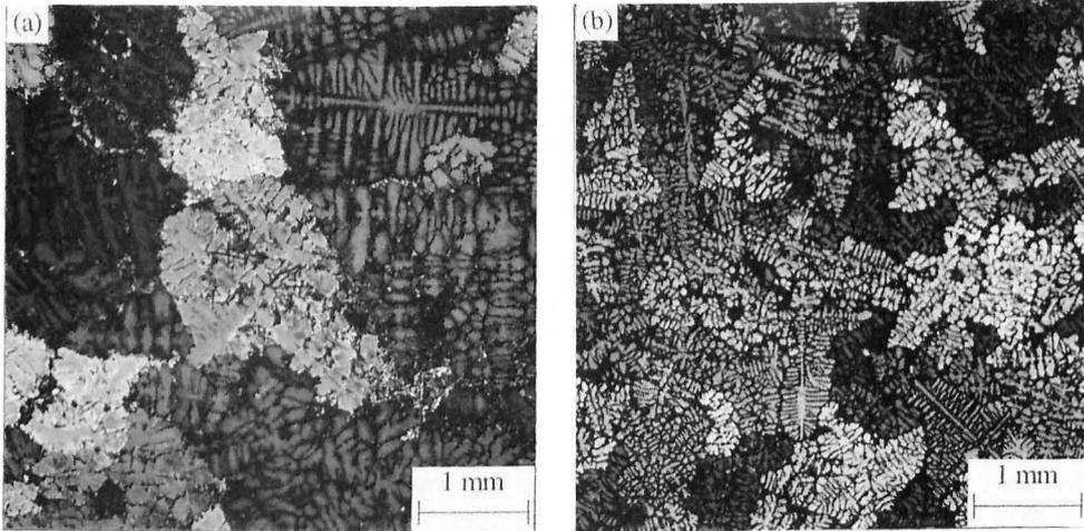
Figure 5. Micrographs showing the effect of cooling rate in commercial Al- 7% Si. a) 0.3 K/s and b) 3 K/s.
