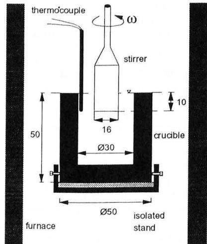
Figure 1. Schematic illustration of the rheological setup.
