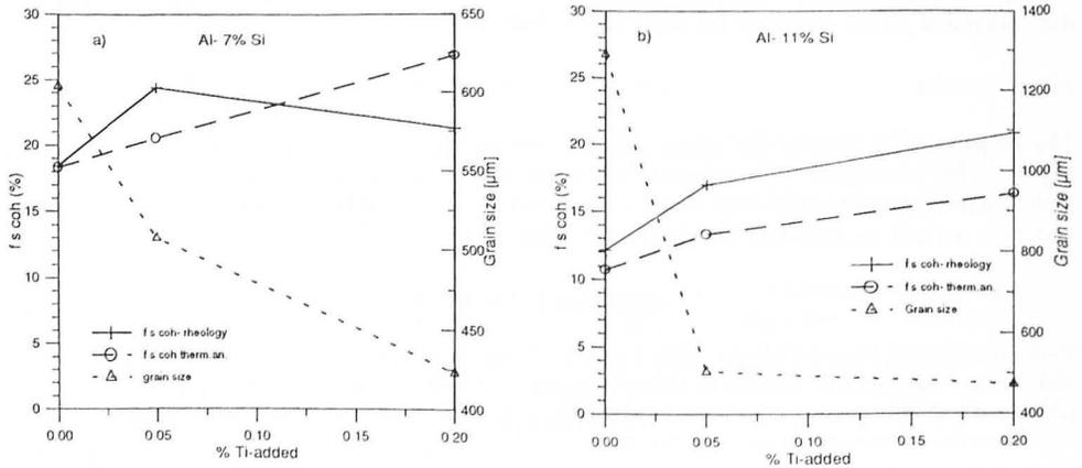
Figure 2. Effect of grain refinement on the coherency point, measured by thermal analysis and rheology, and grain size in a) Commercial Al-7%Si and b) Commercial Al-11%Si. [0.7 K/s]
