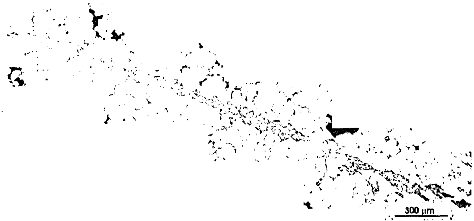
Fig.7 The primary phase \text{Al}_6\text{Mn} in alloy II-2
