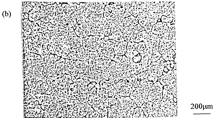
Figure 1. Typical micrographs from material (a) water quenched and (b) slow cooled (30°C/hour) from the homogenisation temperature.
