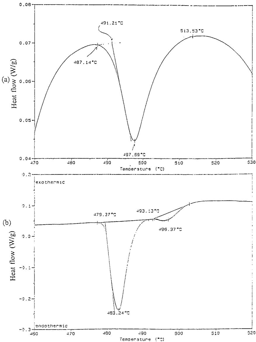
Figure 2. Typical D.S.C. traces produced from material (a) water quenched and (b) slow cooled (30°C/hour) from the homogenisation temperature.
