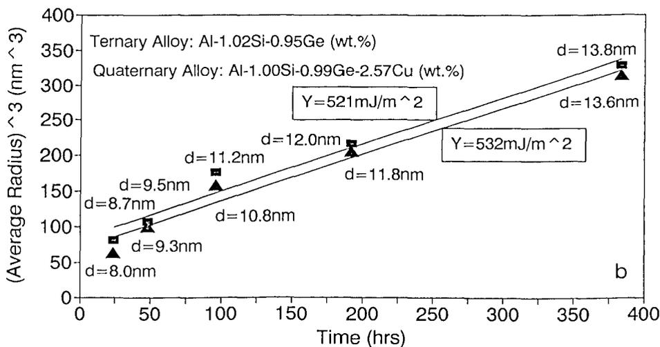
Figure 2. Coarsening behavior of diamond SiGe precipitates in alloys 1 and 2 aged at 160°C. (a) Average diameters. (b) Relationship between cube of average radii and aging time, interfacial energy values (Y).
