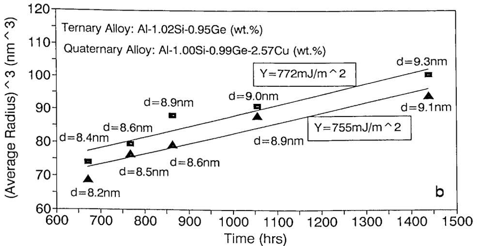
Figure 1. Coarsening behavior of SiGe diamond precipitates in alloys 1 and 2 aged at 120°C. (a) Average diameters. (b) Relationship between cube of average radii and aging time, interfacial energy values ( $\gamma$ ).
