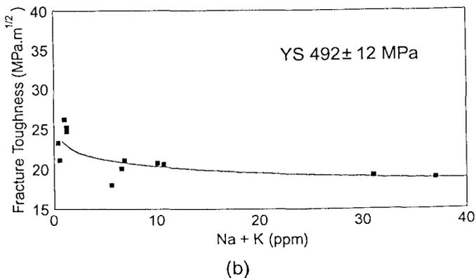
Figure 1: S-L Fracture Toughness versus AMI content for yield strengths of (a)  $440 \pm 12$  MPa (b)  $492 \pm 12$  MPa. Alloy composition 2.0 wt% Li, 2.4 wt% Cu, 0.1 wt% Zr
