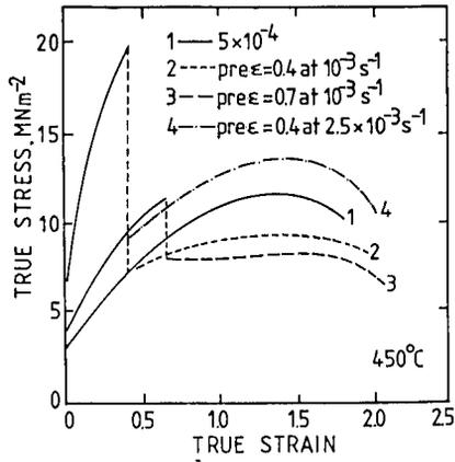
Fig.4 Effect of rapid pre-straining on stress versus strain.
