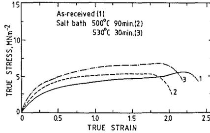
Fig.6 Effect of pre-annealing on stress versus strain at 530°C and  $5 \times 10^{-4} \text{ s}^{-1}$ .
