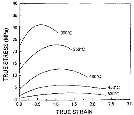
Fig.2 Stress versus strain for strain rate of  $2 \times 10^{-4} \text{ s}^{-1}$ .
