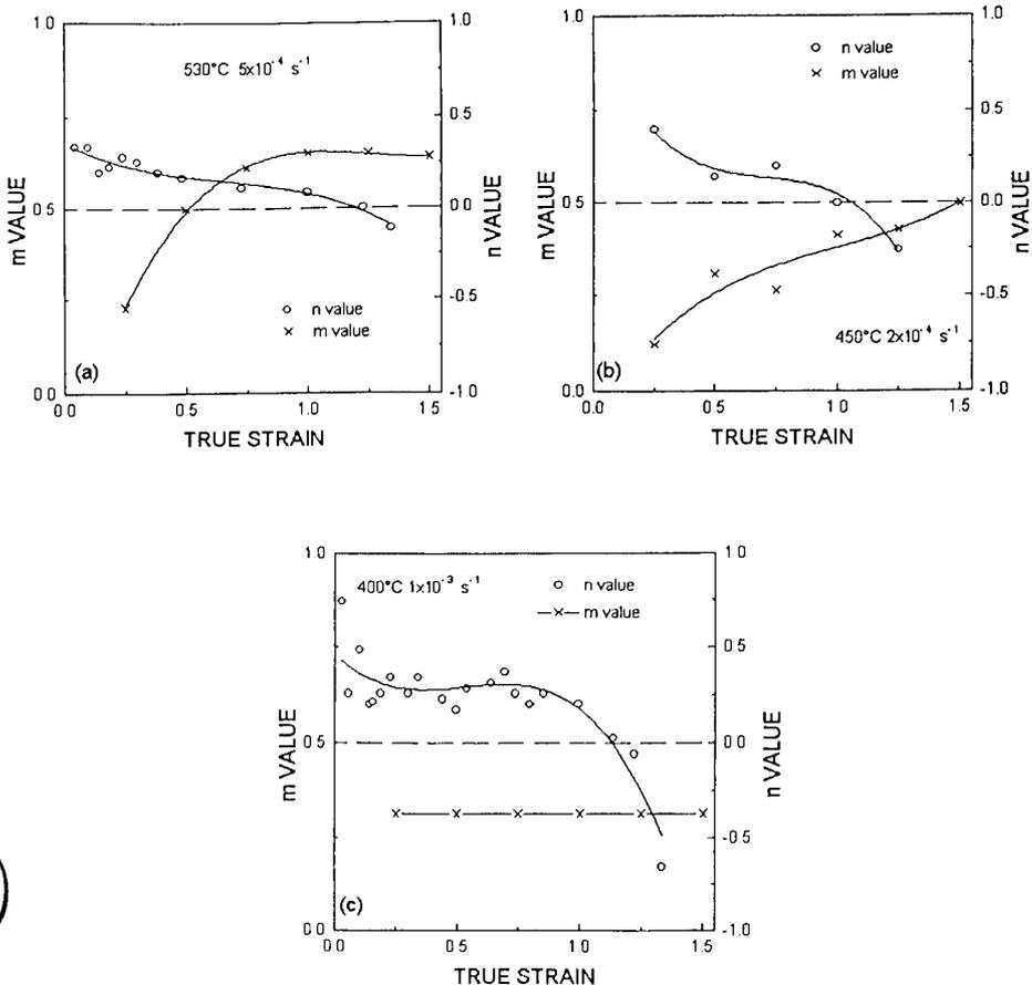
Fig.3 Variation of  $m$  and  $n$  with strain
