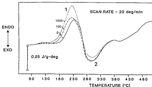
Figure 1. DSC Patterns for Unstretched 2090 Sheet Aged 24 Hours at 163°C and Exposed to 107°C for the Hours Indicated.
