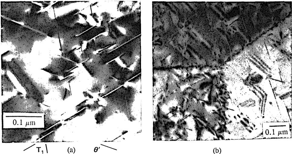
Figure 3. Transmission electron micrographs showing (a)  $T_1$  and  $\theta'$  matrix precipitates, and (b) grain boundaries with no pfz nor coarse, equilibrium precipitates (Courtesy of F.W. Gayle, NIST).
