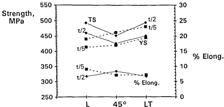
Figure 2. Variation in In-Plane Tensile Properties at the Mid-Plane (t/2) and Near-Surface (t/5) Locations for 3.8 cm Al-2.7Cu-1.5Li-0.3Mn-0.1Zr Plate.
