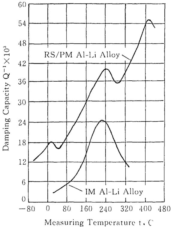
Figure 1. Variation of damping capacity with ascending temperature in the Al-Li-Cu-Mg-Zr alloys (solution treated for 1 hr at 520°C and natural aging). Frequency of vibration = 19.8 Hz at room temperature. Amplitude of vibration = 0.20mm.
