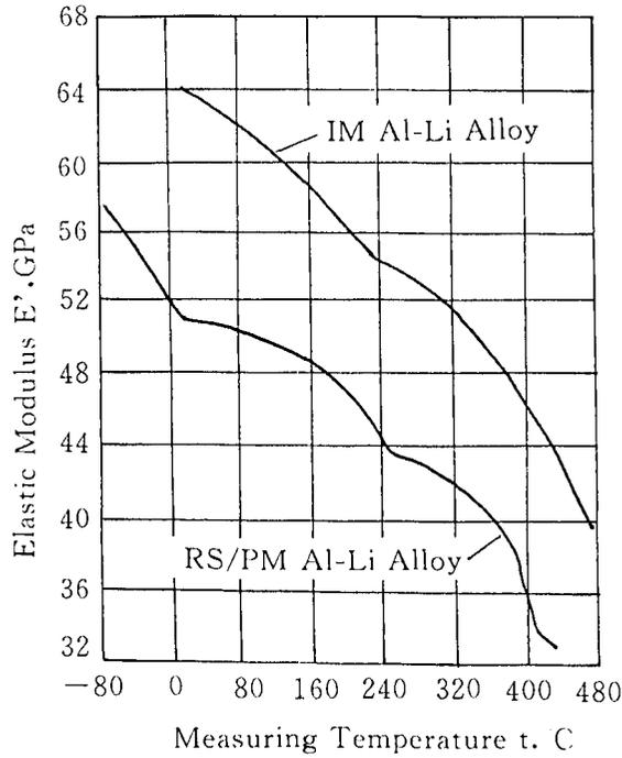
Figure 2. Variation of elastic modulus  $E'$  with ascending temperature in the Al-Li-Cu-Mg-Zr alloys (solution treated for 1 hr at 520°C and natural aging). Frequency of vibration=19.8 Hz at room temperature. Amplitude of vibration=0.20mm.
