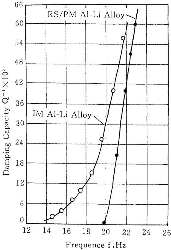
Figure 3. Variation of damping capacity with frequency of resonance in the Al-Li-Cu-Mg-Zr alloys (solution treated for 1 hr at 520°C and natural aging). Amplitude of vibration=0. 20mm.
