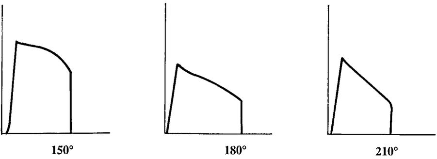
Figure 1 Engineering stress - engineering strain curves (schematic) for 8090-T8 stretched 3% and 7% before ageing in the temperature range 150-210°C
