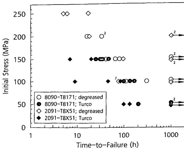
Figure 3. Time-to-failure data for plate material of the alloys 8090-T8171 and 2091-T8X51. Short transverse tensile specimens which were degreased or cleaned in an alkaline detergent were permanently immersed in an aqueous chloride-carbonate-bicarbonate solution under constant load conditions. Numbers indicate the numbers of specimens tested.
