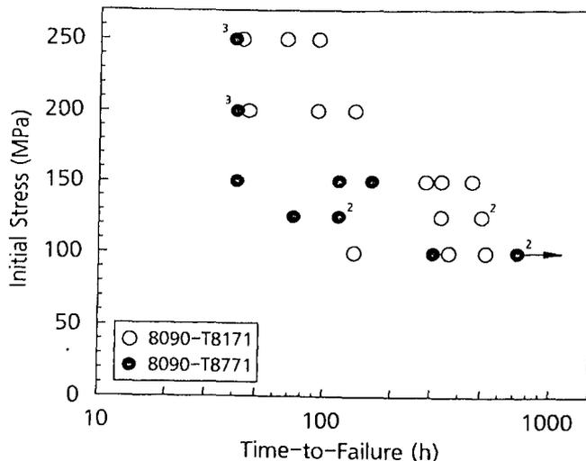
Figure 1. Time-to-failure data for 8090 plate material in the tempers T8171 and T8771. Short transverse tensile specimens were alternately immersed in 3.5% NaCl solution according to ASTM G44. Numbers indicate the numbers of specimens tested.
