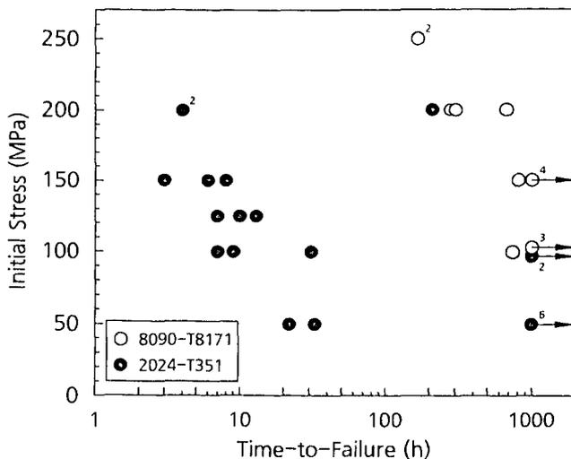
Figure 4. Time-to-failure data for plate material of the alloys 8090-T8171 and 2024-T351. Short transverse tensile specimens were permanently immersed in substitute ocean water under constant load conditions. Numbers indicate the numbers of specimens tested.
