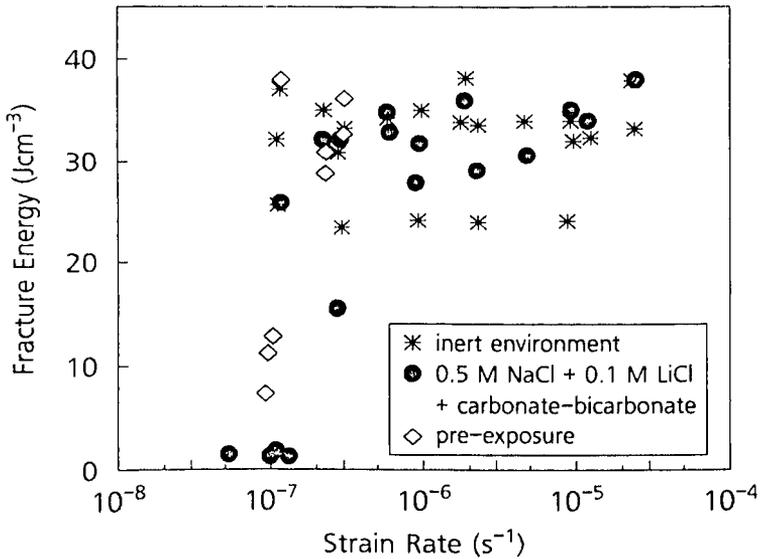
Figure 6. Results of slow strain rate tests for 8090-T8171 plate using an aqueous chloride-carbonate-bicarbonate solution.
