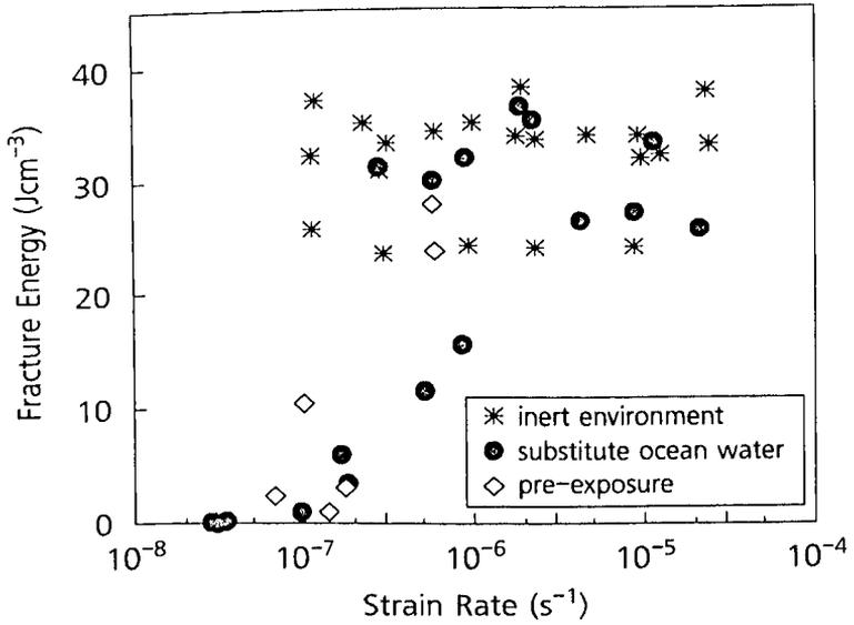
Figure 5. Results of slow strain rate tests for 8090-T8171 plate using substitute ocean water.
