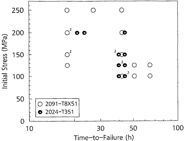
Figure 2. Time-to-failure data for plate material of the alloys 2091-T8X51 and 2024-T351. Short transverse tensile specimens were alternately immersed in 3.5% NaCl solution according to ASTM G44. Numbers indicate the numbers of specimens tested.
