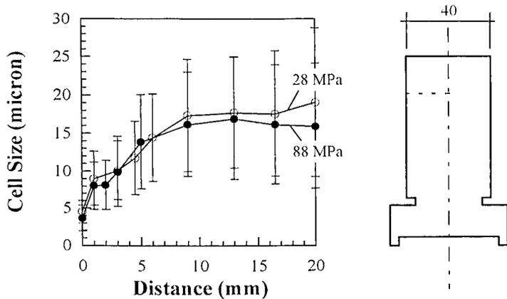
Figure 3. The results of dendrite cell size measurements on two castings squeeze cast at 29 MPa (a) and 88 MPa (b) respectively. The corresponding positions of the measurements are indicated by the horizontal dashed line in the sketch of the casting.
