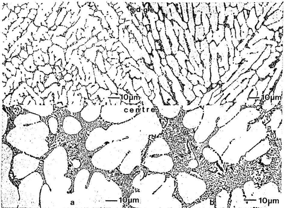
Figure 2. Optical micrographs of two castings of AA603 Al alloy squeezed with pressure of 29 MPa (a) and 88 MPa (b) respectively.
