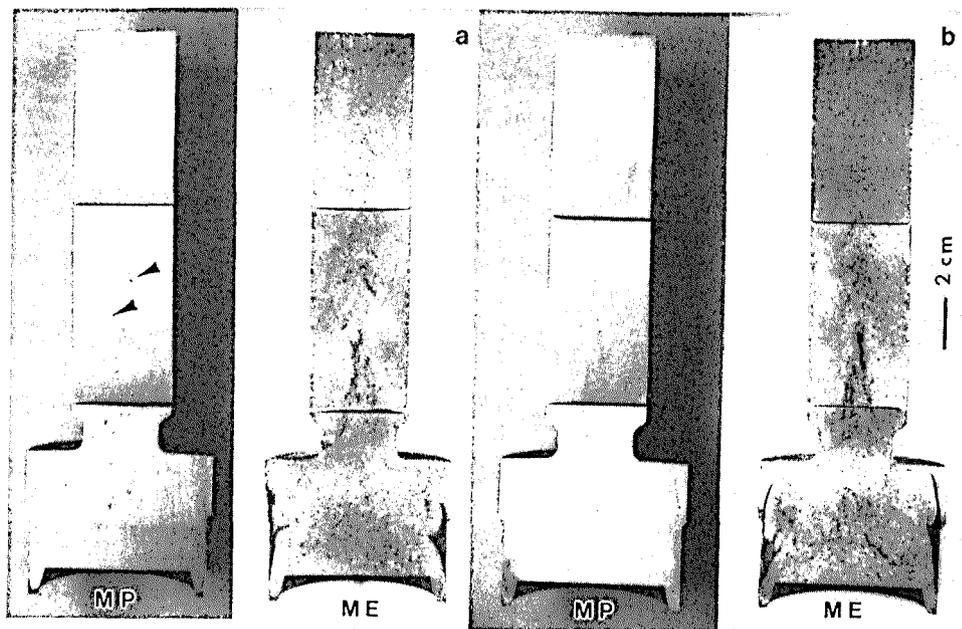
Figure 5. Photographs of two sectioned cylindrical castings of alloy AA603 with long biscuits squeezed at 29 MPa (a) and 70 MPa (b) respectively. "MP": after mechanical polishing, and "ME": after macro-etching. Arrows indicate fine porosity.
