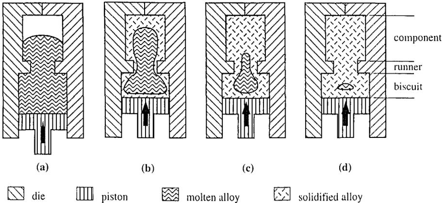
Figure 1. Schematic illustration of mould filling and solidification sequence in the indirect squeeze casting method.
