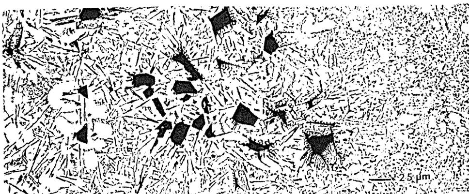
Figure 8. Optical micrograph showing coarse Si crystals found in a cylindrical casting of AA603 squeezed at 82 MPa.
