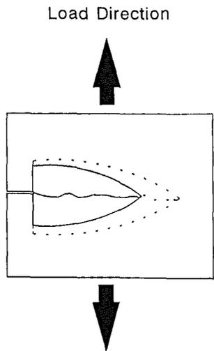
Figure (6): Growth of the delamination zone with crack length.
