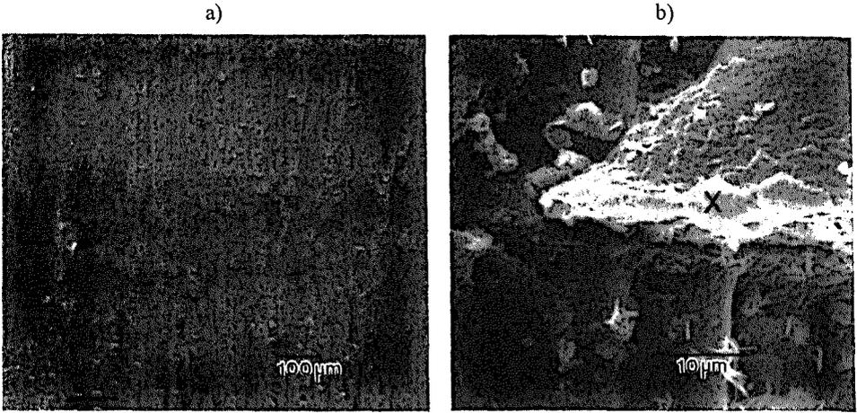
Figure 5: Traces of fatigue crack path on the surface of the delamination zone a) for a thin resin-rich layer and b) for a thick resin-rich layer with resin remaining attached to the surface (X).
