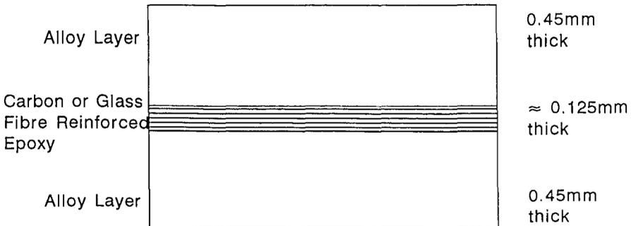
Figure 1: The 2-1 configuration of the laminates
