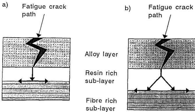
Figure 4: Schematic of crack path through a) a thin resin-rich layer and b) a thick resin-rich layer.
