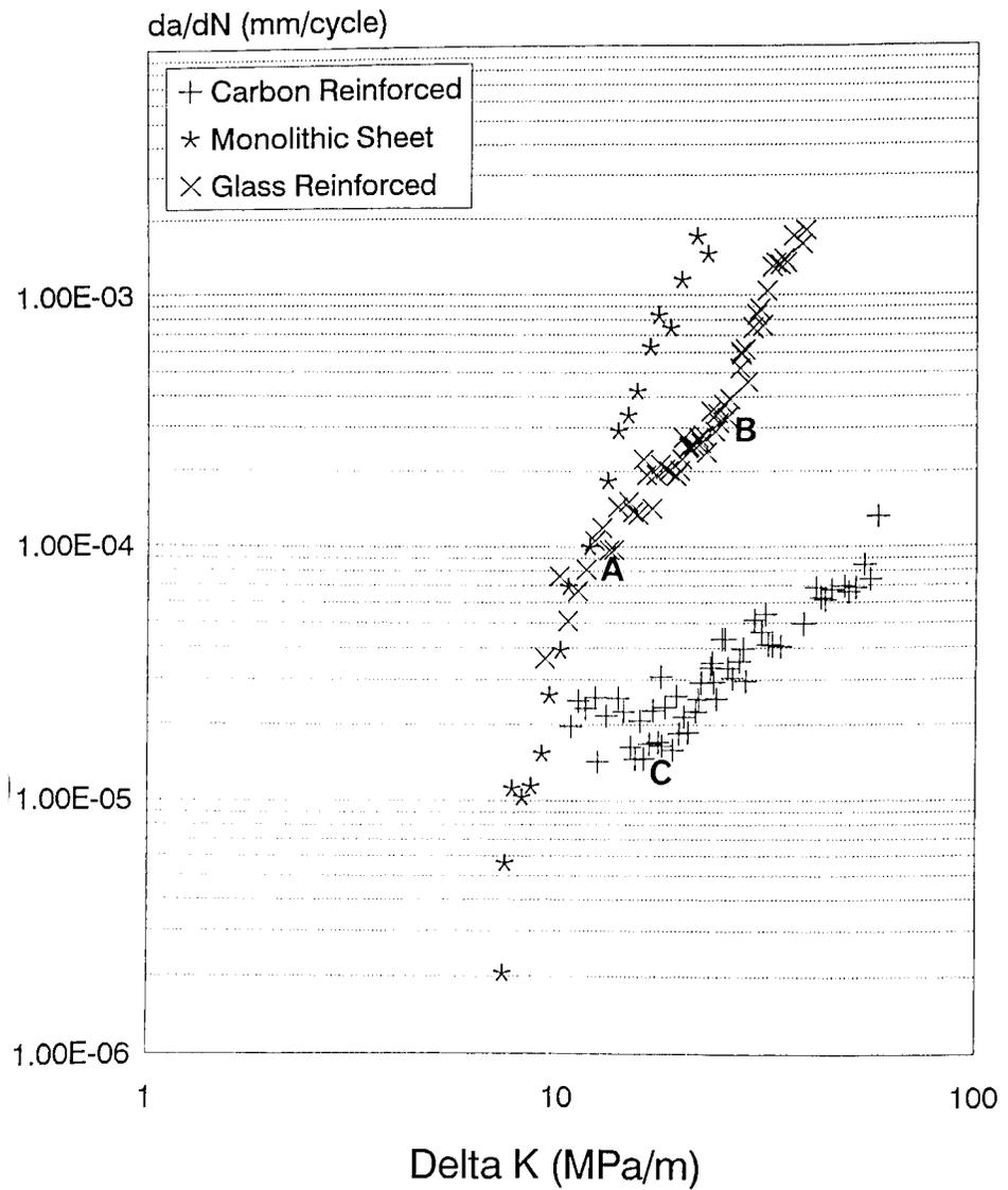
Figure 7: Fatigue crack growth rates for carbon and glass reinforced laminates and monolithic sheet tested at  $R=0.1$ , initial  $\Delta K \approx 9 \text{ MPa}\sqrt{\text{m}}$ ,  $f = 20\text{Hz}$ .
