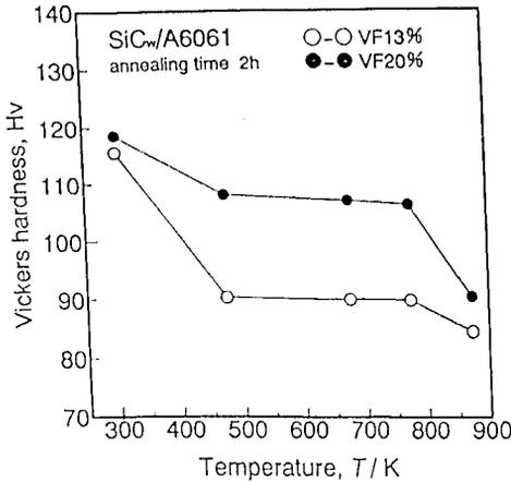
Fig. 1. Hardness changes of SiCw/6061 Al composites after isochronal annealing for 2h at various temperatures.
