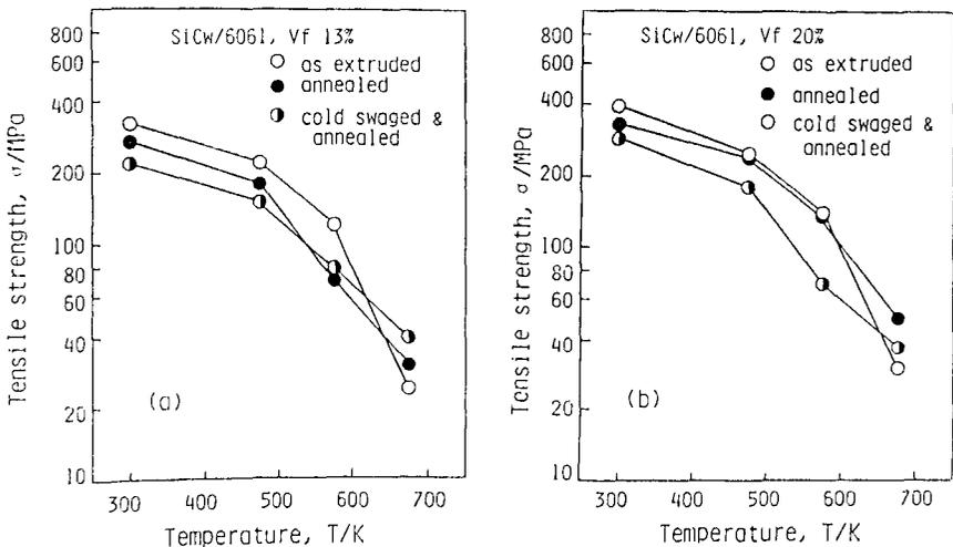
Fig. 7. Tensile strength at various temperatures of SiCw/6061 Al composites with and without directional annealing. (a) Vf13% and (b) Vf20%.
