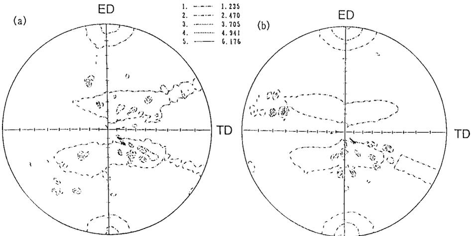
Fig. 6.  $\langle 111 \rangle$  pole figures of the aluminum matrix of directionally annealed composites of SiCw/6061 Al, (a) Vf13% and (b) Vf20%.
