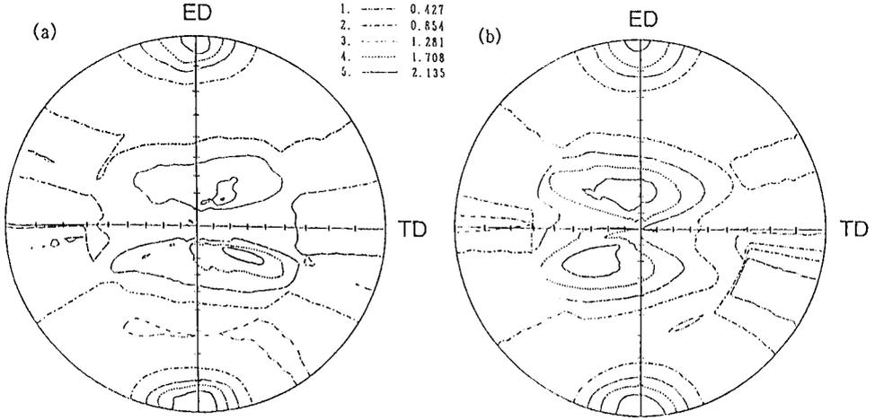
Fig. 5.  $\langle 111 \rangle$  pole figures of the aluminum matrix of as-extruded composites of SiCw/6061 Al, (a) Vf13% and (b) Vf20%.
