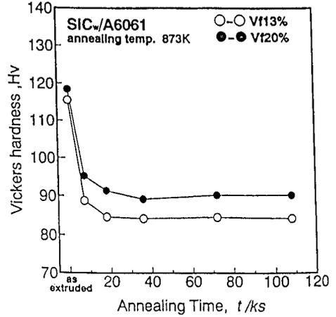
Fig. 2. Hardness changes of SiCw/6061 Al composites on annealing at 873K.
