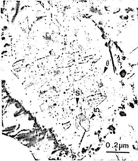
Figure 2 Three phases \Omega , s' , and \theta' formed in 2009M P/M alloy.
