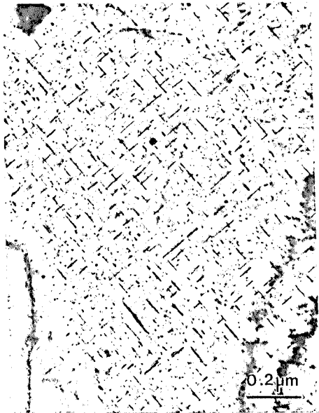
Figure 9. The s' size and distribution in the 2009M/SiC p thermally exposed 500 hours at 150°C after peak aging.
