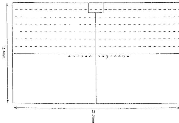
Figure 2. Surface removal followed by blind-hole drilling to the centre of the specimen
