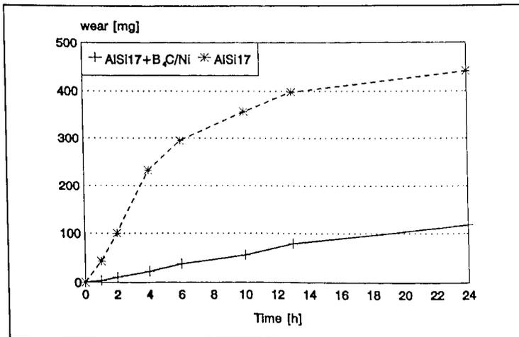
Figure 8. Cavitation erosion of as cast and laserfused AISi17 in comparison
