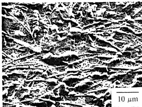
Figure 2. AlSi17 +  $B_4C$ : See left track (Fig. 1) structure of the central zone: small partly remelted ceramic particles, rapidly quenched aluminum-silicon and needle like phases
