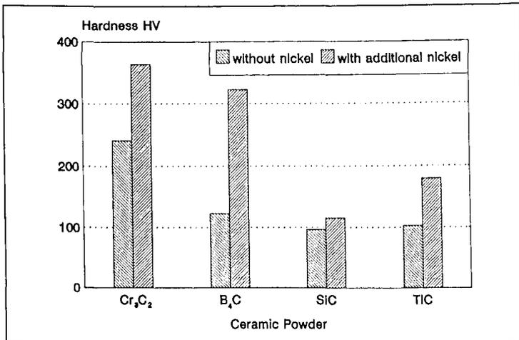
Figure 5. Hardness of the central zones after laser surfacing with different ceramics
