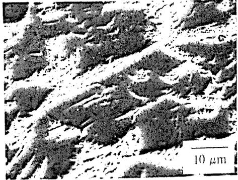
Figure 4. AlSi17+B<sub>4</sub>C: See right track (Fig. 1): Cermet like structure in the central zone
