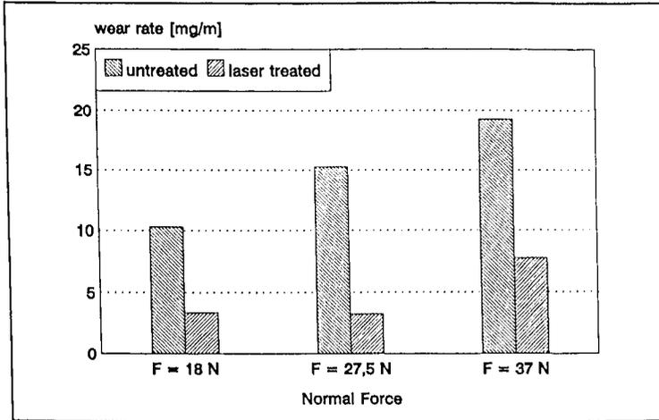
Figure 7. Grooving wear against Flint 80 of as cast and laserfused AISi 17
