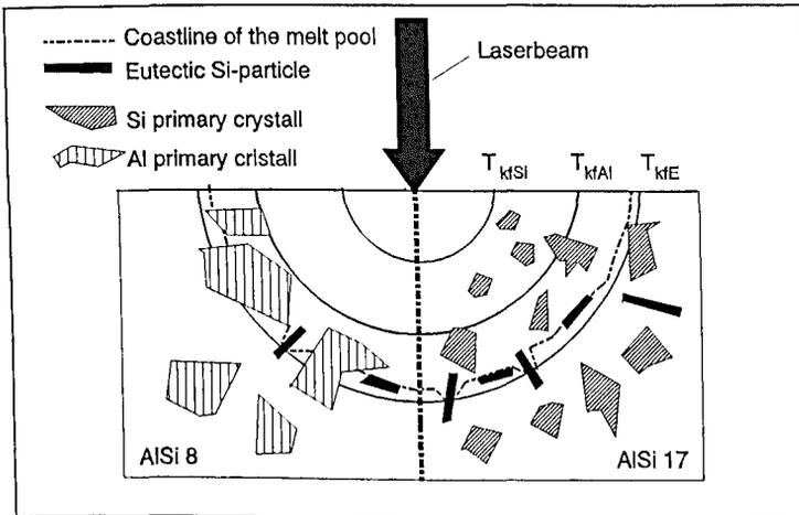
Figure 9. Rapid heating of multiphase material, schematic (e.g. Al-Si-alloy, left: hypoeutectic, right: hypereutectic). The melting temperatures ( $T_{kf}$ ) of the different microstructure elements are important.
