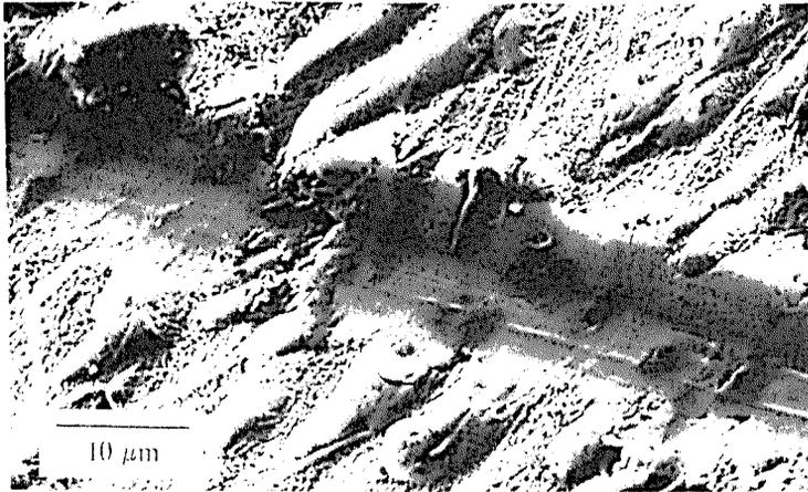
Figure 6. Scratchgroove in a central zone containing  $B_4C$ , microcutting predominates
