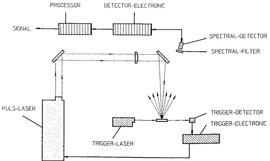
Figure 5. Diagram of the detection process for analytical identification of shredder scrap [3]
