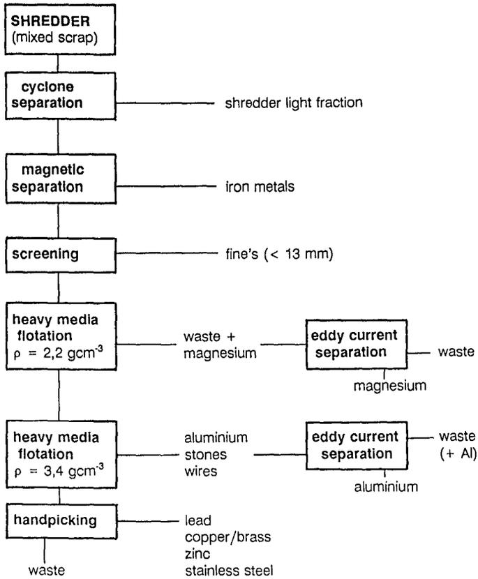
Figure 8. Flow diagram of presently carried out separation for the recycling of metals from automobile shredder.
