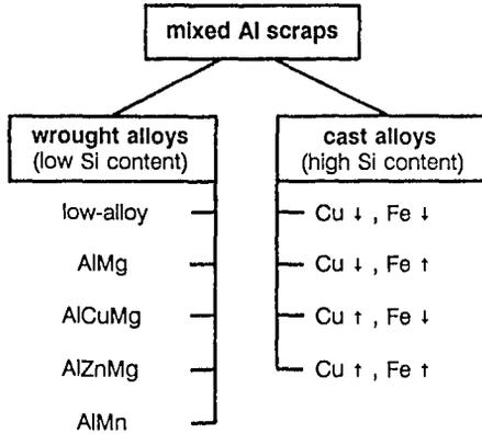
Figure 6. Scheme for sorting of mixed Al-scrap. The separation of five wrought and four casting alloy types is possible by laser aided identification of alloy constituents.
