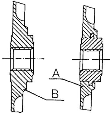
Figure 11. Example for recycling oriented product design of a belt-pulley for washing machines, after [7].
