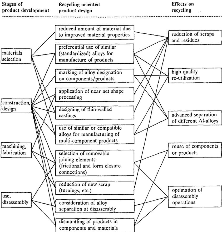
Figure 12. Examples for recycling-oriented design of aluminium products including the consequences for recycling if considered in product development.
