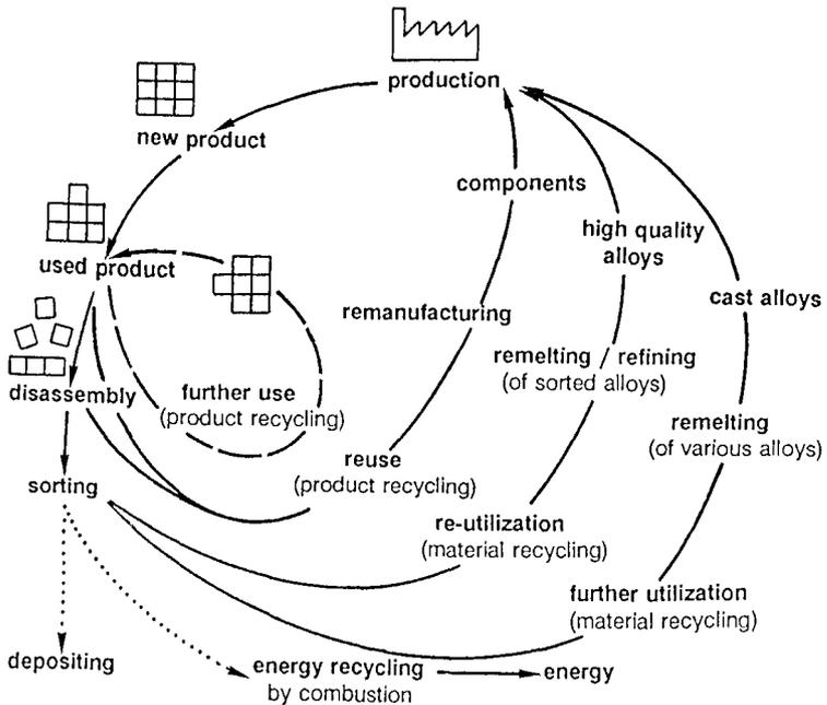
Figure 3. Life cycle of aluminium products and materials.
