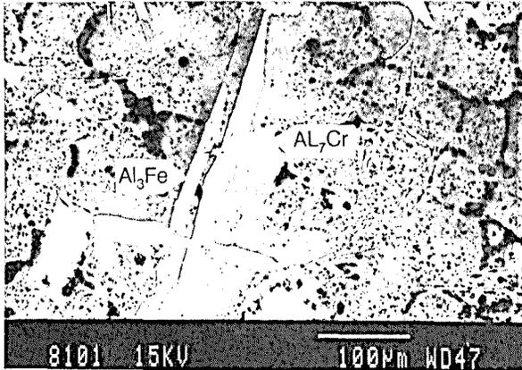
Figure 7. Al-5wt%Li (model alloy): formation of undesired phases (Al<sub>3</sub>Fe and Al<sub>7</sub>Cr) due to alloy contamination by Fe and Cr [SEM-micrograph].
