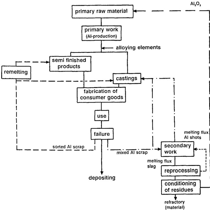
Figure 10. Flow diagram for the material recycling of aluminium; Re-utilization of sorted Al scrap for manufacturing of high quality castings or semi finished products and further utilization of mixed Al scrap for production of castings.
