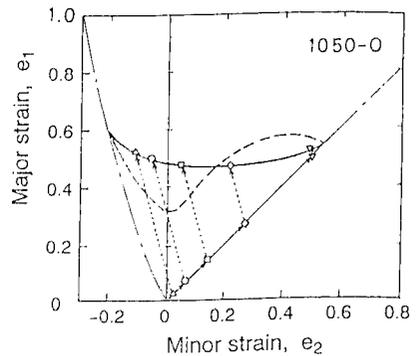
Fig. 3 Forming limit strains with Strain path-2.
