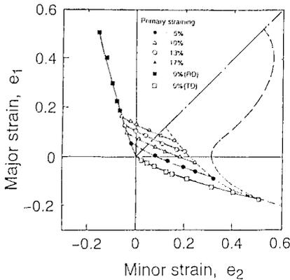
Fig. 2 Forming limit strains with Strain path-1.
