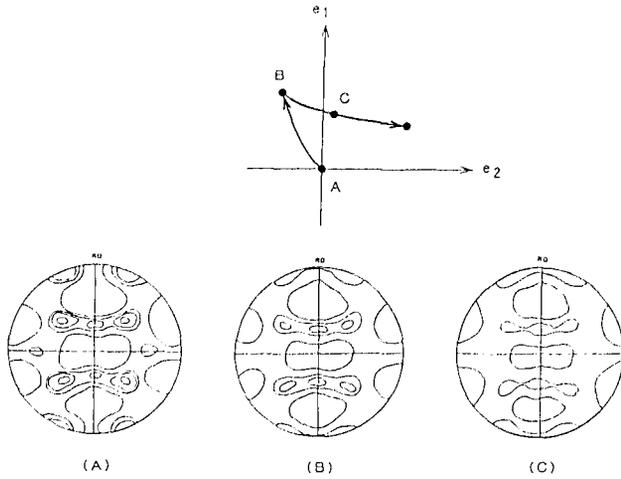
Fig. 4 (111) pole figures of aluminum deformed with Strain path-1.
