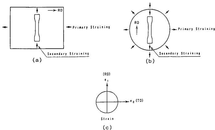
Fig. 1 Relations between the primary and the secondary stage deformation in Strain path-1 (a) and Strain path-2 (b). Directions of the strains (c).
