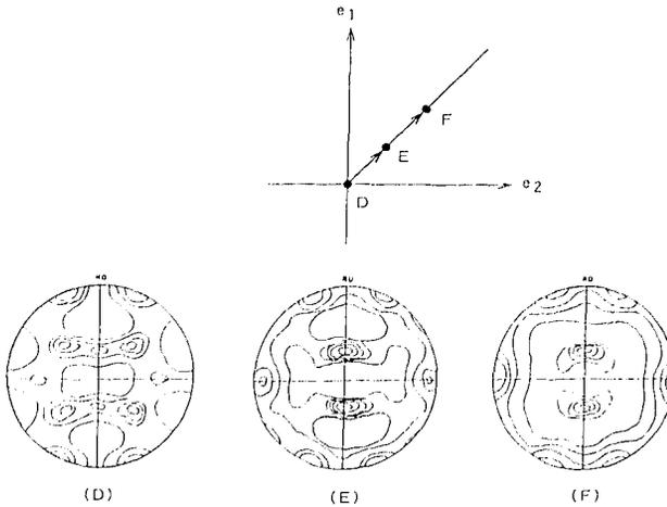
Fig. 5 (111) pole figures of aluminum deformed with the primary stage of Strain path-2.
