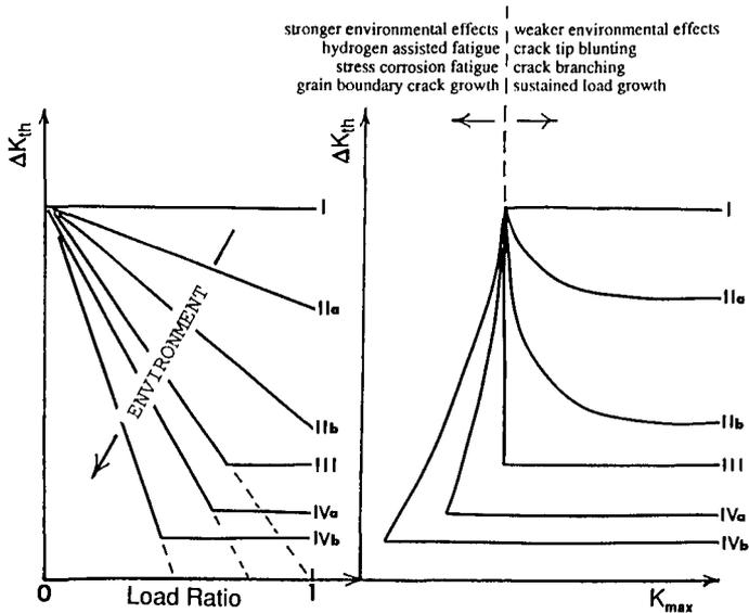
Figure 4. Schematic explanation of the overall fatigue mechanisms to indicate the four main classifications in terms of (a)  $\Delta K_{th}$  vs  $R$ , and (b)  $\Delta K_{th}$  vs  $K_{max}$ , along with the regions affected by the environment.
