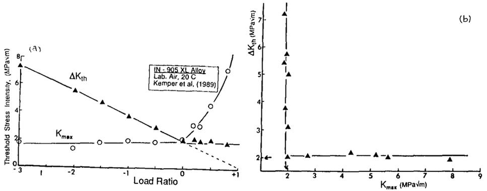
Figure 1. (a) Variation of  $\Delta K_{th}$  and  $K_{max}$  with load ratio  $R$  for a IN-905 Aluminum alloy in lab. air, and (b) a replot of (a) as  $K_{max}$  dependence on  $\Delta K_{th}$ .
