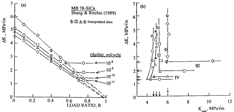
Figure 6. Class-IV MB-78-SiCp aluminum composites data extended to higher crack growth rates showing the transition from Class-IV to Class-III; in the form of (a)  $\Delta K_{th}$  vs R, and (b)  $\Delta K_{th}$  vs  $K_{max}$ .
