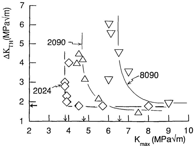
Figure 2.  $\Delta K_{th}^*$  and  $K_{max}^*$  plot comparing the two planar slip deforming Al-Li alloys (8090 & 2090) with a conventional homogeneously deforming 2024-T3 alloy.
