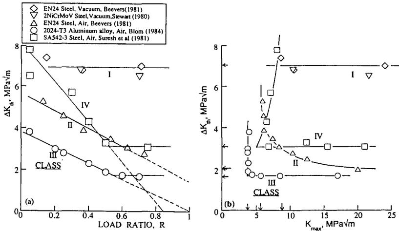
Figure 5. Experimental results showing the different class of fatigue behavior in terms of (a)  $\Delta K_{th}$  vs R, and (b)  $\Delta K_{th}$  vs  $K_{max}$ . The results were taken from aluminum and steel alloys.
