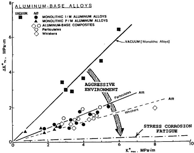
Figure 3. Illustrations of the role of environment affecting the critical stress intensity parameters,  $\Delta K_{th}^*$  and  $K_{max}^*$ , for the aluminum-base composites. For comparison, vacuum data of monolithic alloys is shown.
