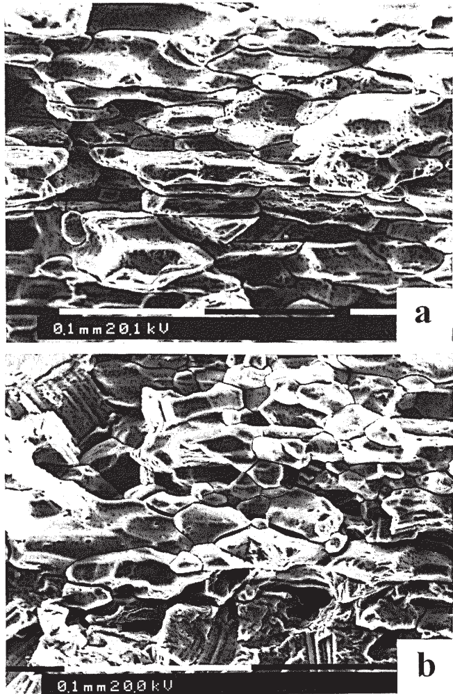
Figure 5: Scanning electron fractographs of 8090-T81 specimens which were strained in an aqueous solution of 0.5 M NaCl + 0.1 M LiCl + 0.05 M NaHCO 3 + 0.05 M Na 2 CO 3 (a) and in substitute ocean water (b), showing attacked grain boundaries.
