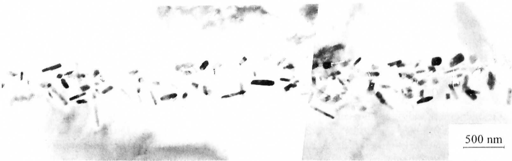
Fig. 3 : band of precipitates observed after a 10 s holding at 400°C
