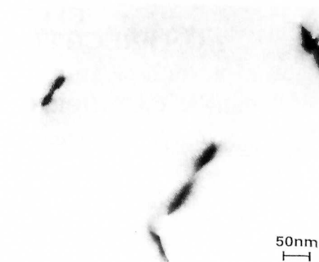
FIGURE 2. \langle 110 \rangle_{\alpha} BF TEM image of the AQ microstructure of alloy 1.
