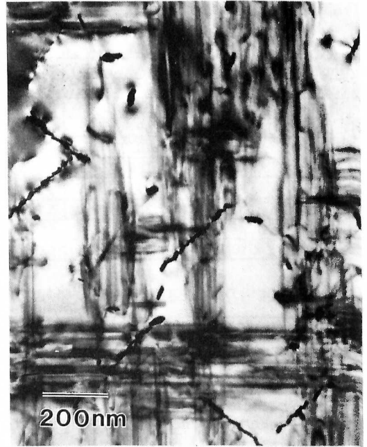
Figure 4. TEM bright field image showing the In-containing alloy. B=[001]_{Al}
