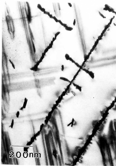
Figure 5. TEM bright field micrograph showing the La containing alloy. Note the criss-cross nature of the S' corrugations and the strain contrast at the precipitate/matrix interface. B=[001]_{Al}
