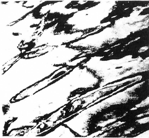
Fig.7. TEM of the sample deformed 39% at 3996\text{s}^{-1}
